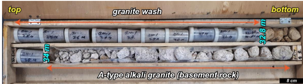
Figure D1: Photograph showing drilled core. The lowermost of the unconsolidated sediments, the granite wash, directly overlies bedrock. Cosmogenic ^{10}\text{Be} - ^{26}\text{Al} isochron dating samples are taken from this granite wash.
