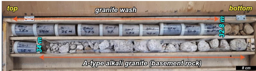
885 Figure DE1: Photograph showing drilled core. The lowermost of the unconsolidated sediments, the granite wash, directly overlies bedrock. Cosmogenic ^{10}\text{Be} - ^{26}\text{Al} isochron dating samples wereare taken from this granite wash.
