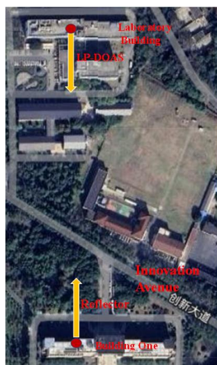
Figure 14 LP-DOAS telescope, reflector position (optical path of 700m, from © Google Maps)
