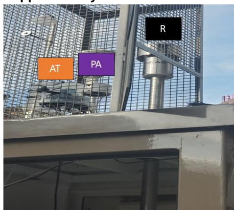
Supplementary Figure 1: AT= Atmotube Pro sensors in a makeshift cover to shield rain; PA=Purple Air sensor; R= Reference FIDAS monitor inlet.
