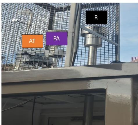
Supplementary Fig.1: AT= Atmotube Pro sensors in a makeshift cover to shield rain; PA= Purple Air sensor; R= FIDAS reference monitor inlet
