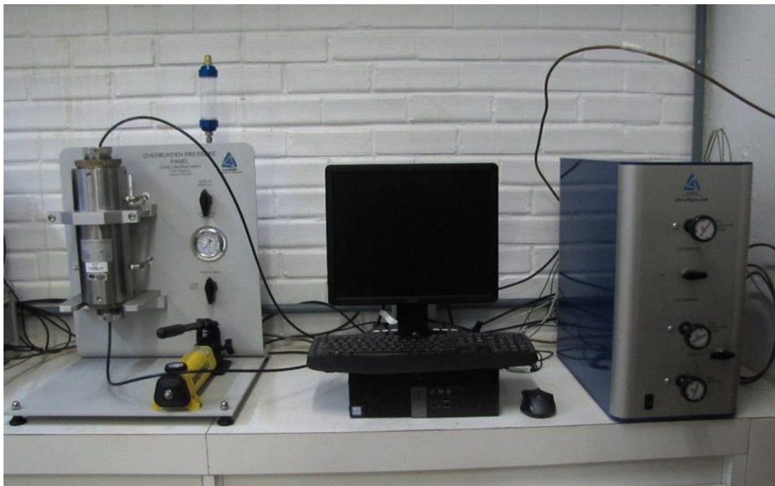
57 58 Figure S2. Ultra-Perm 610 gas permeameter with pressure sample saturator (Core Lab 59 Instruments).
