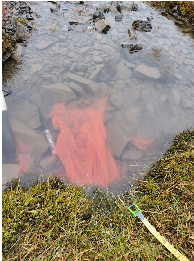
Figure B1. Rhodamine tracer emerging at the groundwater spring on the downslope side of the hillslope area in Endalen valley during tracer experiments conducted in September 2022. The liquid tracer was injected 2 m uphill in groundwater at approximately 0.5 m depth. First arrivals were observed only after a few minutes after injection.
