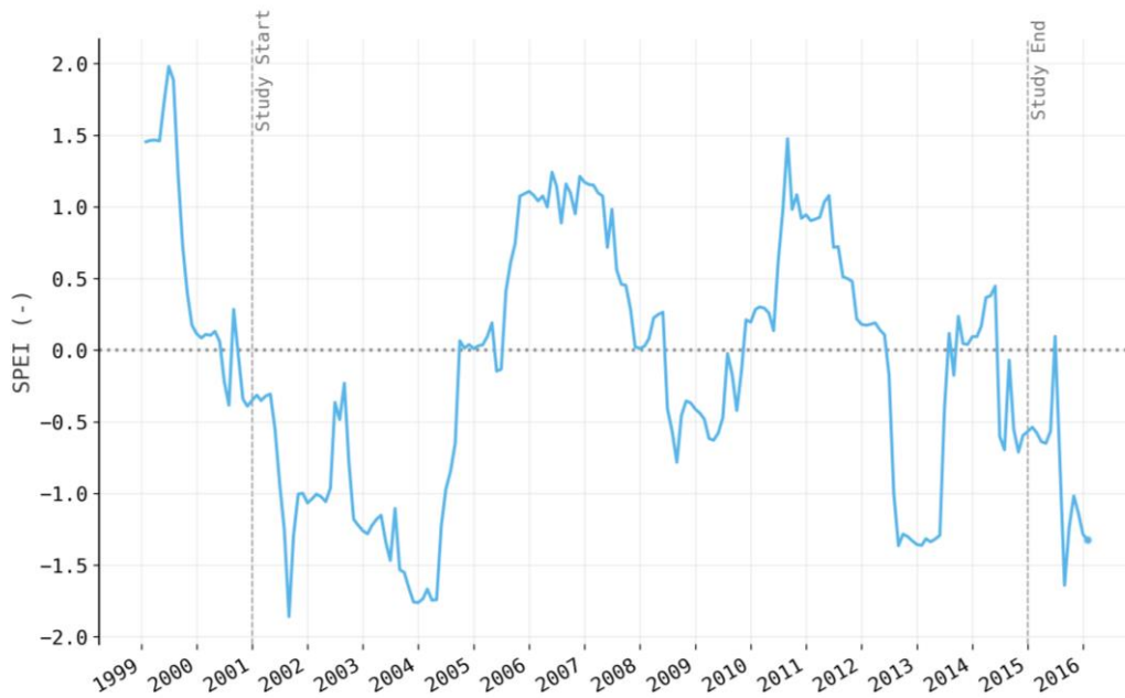
Figure 3 The average 12-month Standardized Precipitation Evaporation Index (SPEI) in the Bhima basin. Derived from the CHELSA-W5E5 v1.0 dataset (Karger et al., 2022).
