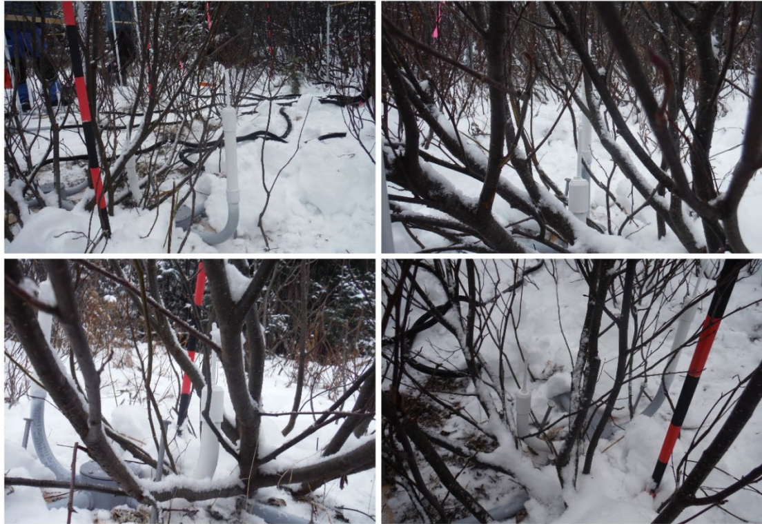
30 Figure S1. Photographs of the S325 and S485 sensors during installation on December 2 nd 2020. The S325 sensor is at the center of the shrub while the S485 sensor is near its edge. The nails were hammered into the ground shortly afterwards to ensure they would not perturb radiation transfer. The snow visible here melted entirely on December 25 th (Figure 6). The color stripes on the snow stake are 10 cm high.
