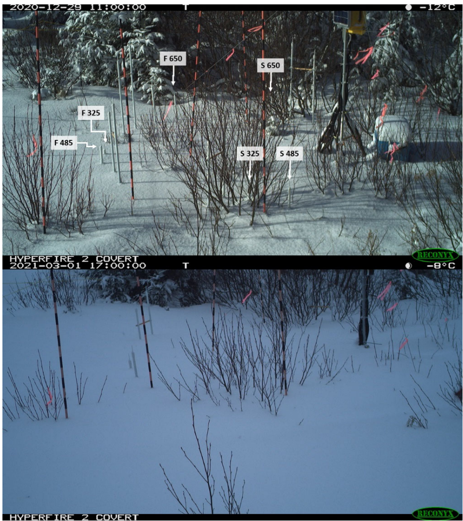
Figure 2. Photographs of the site showing the positions of the sensors. (top) On December 29, 2020, when no sensor was covered by snow. The six sensors whose data were used here are indicated. S325, S485 and S650 are in the SHRUB spot at heights of 325, 485 and 650 mm. F325, F485 and F650 are in the FIELD site. (bottom) Same view at peak snow height on March 1 st , 2021, when the six sensors were buried. Note that the snow bent the branches, modifying the branch environment of the S sensors visible on top.
