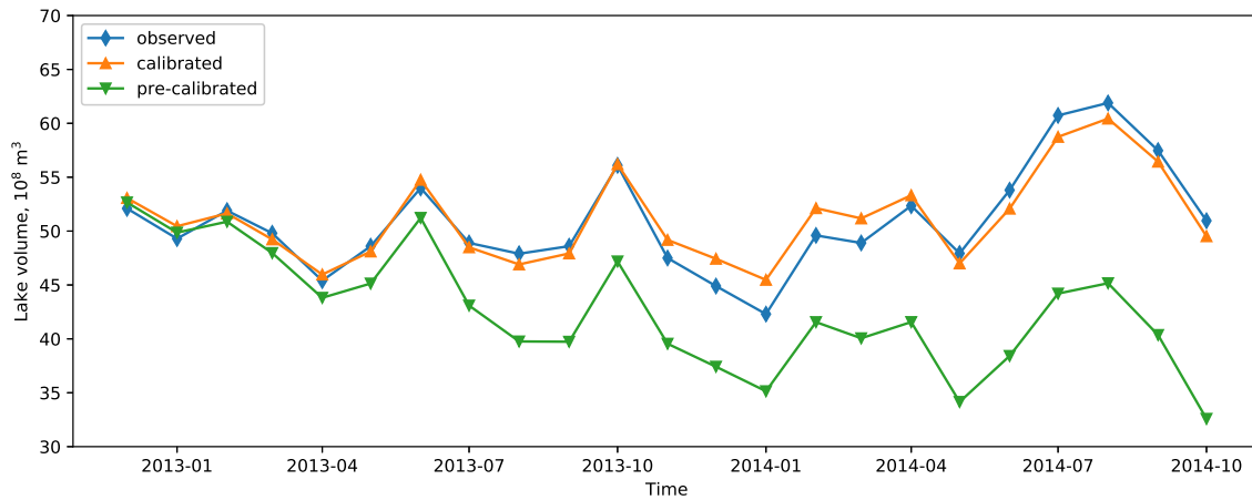
Figure S5. Calibration of mass balance model for lake water. The blue line is the lake volume; the pre-calibrated line lake volume is calculated using mass balance equation and the calculated evaporation rate by Penman equation; the calibrated lake volume is calculated using the mass balance equation and the calibrated evaporation rate.
