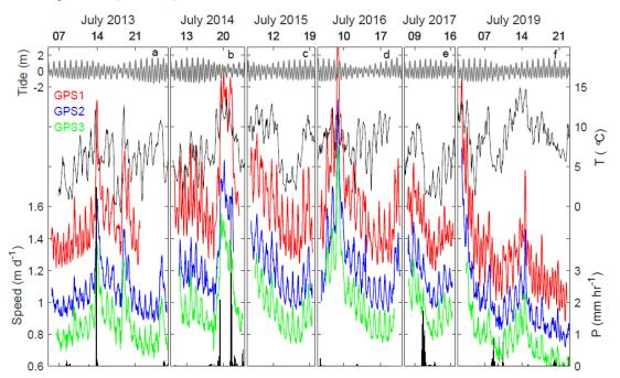
Figure 2: Ice speed at GPS1–3 (red, blue, and green), tidal height (grey), air temperature (black) and precipitation (bar).
