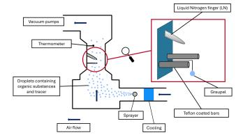
**Figure 2.** Schematic of the wind tunnel. Cooled air transported the generated water droplets containing the compounds into the experimental region (red circle). Red rectangle – the enlarged experimental area shows the three surfaces on which the riming took place: graupel, the liquid nitrogen finger, and Teflon-coated bars.
