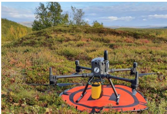
160 161 Figure 3. DJI Matrice 300 RTK equipped with the YellowScan Mapper + in front of the Ridge palsa.
