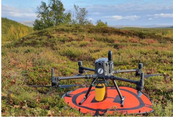
185 186 Figure 3. DJI Matrice 300 RTK equipped with the YellowScan Mapper_+ in front of the Ridge pPalsa.
