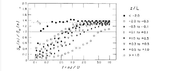
Figure 22. Plot of the ratios of w and u spectral estimates showing approach to the 4/3 ratio required for isotropy.
