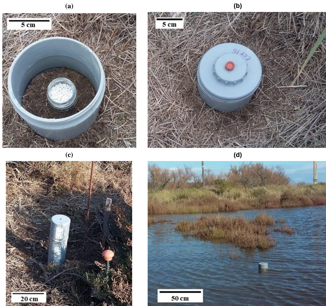
Figure S1. Opaque chambers used to take the measurements of net soil CO 2 and CH 4 fluxes under non-flooded (a and b) and flooded (c and d) conditions. When soil was not flooded, soda lime was placed inside the chamber (a) and then it was hermetically closed (b).
