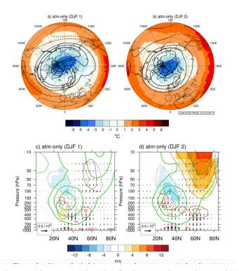
Figure 5: The same as Fig. 4 but for the *atm-only* experiment. a-b) Zonal wind (contours) and temperature (shading) response at 50 hPa for winter 1 and winter 2, respectively. c-d) EP flux (arrows) and divergence (red contours) response along with zonal-mean zonal wind (black contours) and pure climatology (green contours, 2m) in winters 1-2, respectively. Contours and colored area indicate 95% significance according to a Student's t-test.
