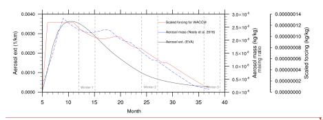
Figure 1: The time series of the original EVA aerosol extinction output (1/km, black curve) and the dry aerosol mass mixing ratio of the volcanic forcing file of Neely et al. (2016) (kg/kg, blue dashed curve) used for deriving the linear scaling coefficient for the conversion of EVA output into WACCM4 input (kg/kg, red curve). The horizontal axis is time (months) from the start of the
