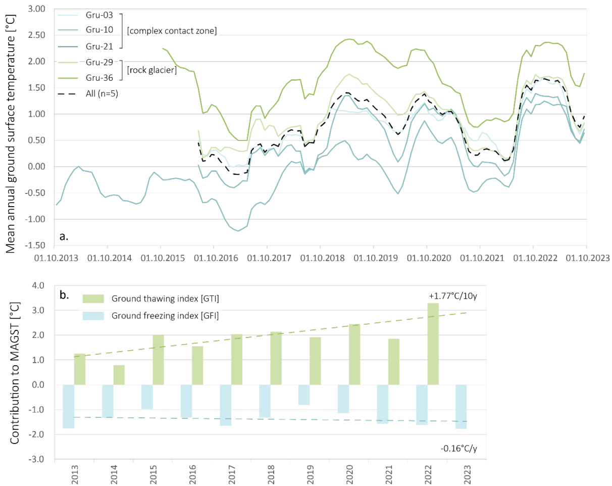
Figure 2: Running MAGST measured on the Gruben rock glacier and complex contact zone (a) and contribution of the ground thawing index (GTI) and ground freezing index (GFI) to the MAGST at Gruben on average (b) (PERMOS, 2023).
