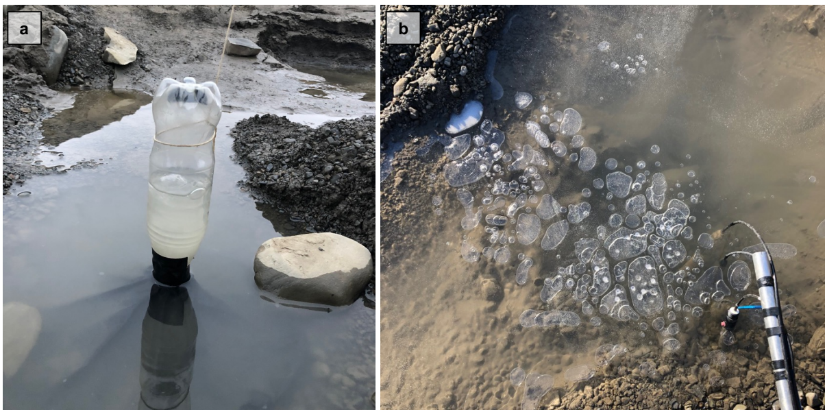
Figure S.2. (a) The bubble trap used to make ebullition measurements, and (b) bubbles resulting from ebullition trapped beneath a thin layer of ice formed on the surface of the GW2 pool during a period with below-freezing temperatures at the end of the summer.
