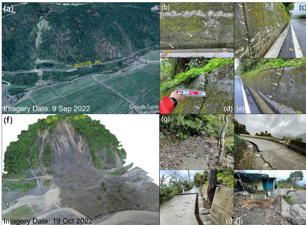
348 Figure 9 (a) Google Earth image before the CL. (b)-(e) Photos from inspection on 27 May 2022. (f) Drone- 349 based 3-dimensional model after the CL. (g)-(j) Photos of crown cracks of the CL.
