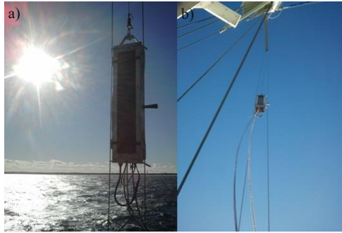
730 Figure B1. The classical aerosol spectrometer on the left panel and the method of device moving between altitude levels during gradient measurements.
