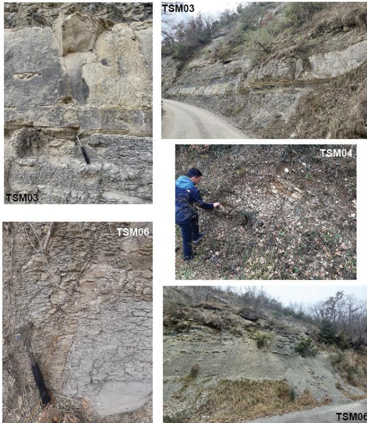
Figure S2. Outcrops of the Marnoso-Arenacea Fm. (TSM03, TSM04 and TSM06). Geological survey provided important information on facies, bedding orientation and geological structures such as faults and cleavage. This allowed us to reinterpret the structures identified in the image logs.
