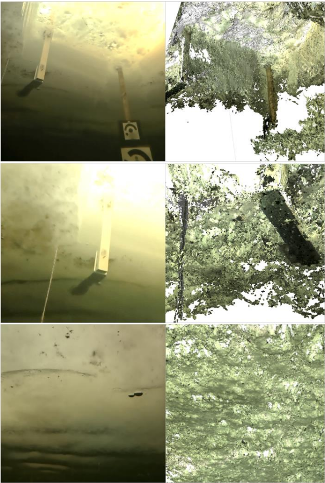
445 Figure 9: Comparison between the raw data (left column) and captures of elevation model of the ice underside (right column). As exact ROV locations weren't known, the input frames and captures of the reconstruction are not taken exactly from the same point.
