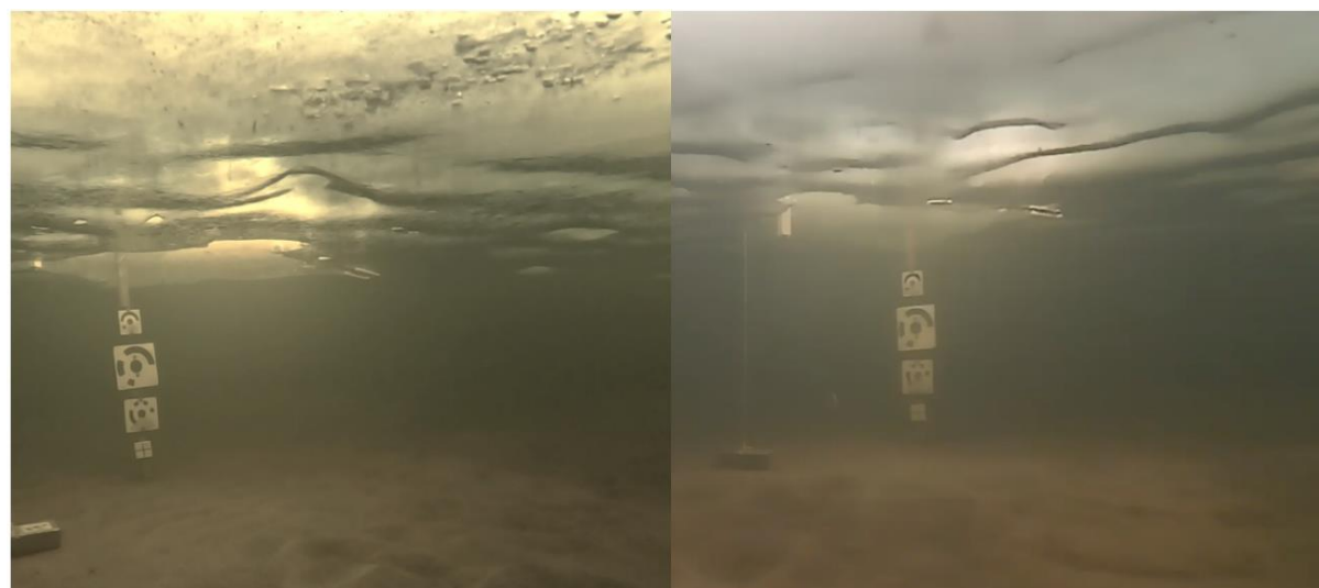
Figure 4: Comparison of image quality between frames taken with GoPro (left) and built-in camera (right) from approximately same location and time step. These two frames presented here have been edited to make them more comparable: the brightness of GoPro frame has been increased and both have been cropped as the GoPro frames were originally taken with portrait orientation and the built-in camera captured with landscape mode. The frames used in the SfM-processing were not cropped. The fields of view differ due to differences in cameras and their orientation.
