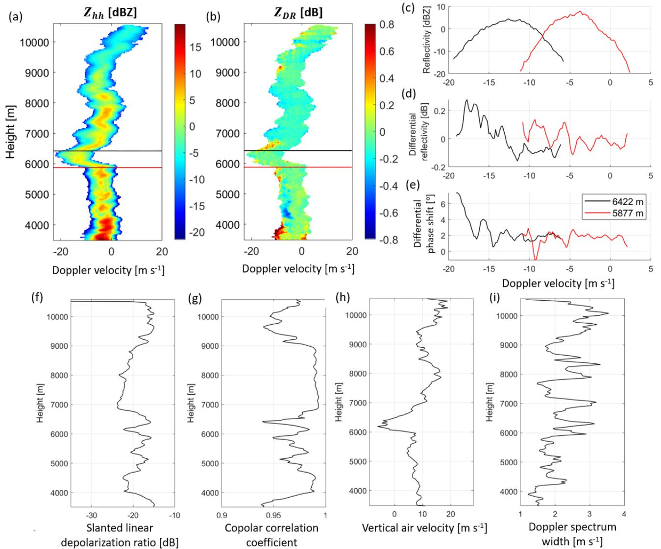
**Figure 27.** 18 June 2021 17:23:47 UTC where the three peaks of  $SL_{DR}$  and troughs of  $\rho_{hv}$  are observed. (a-b) Spectrograms of reflectivity and differential reflectivity (c-e) spectra of reflectivity,  $Z_{DR}$  and  $\Psi_{DP}$  at 5877 m (middle peak) and 6422 m (highest peak) (f-i) profiles of  $SL_{DR}$ ,  $\rho_{hv}$ , vertical air velocity and Doppler spectrum width.
