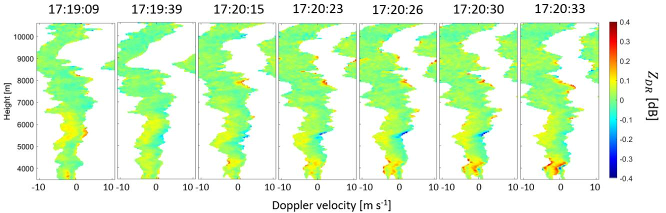
**Figure 22.** Spectral differential reflectivity before and after a strong lightning strike ( $-18$  kA) at 17:20:27 UTC at 5 km cross-range (strike number 92 in Fig. B5).
