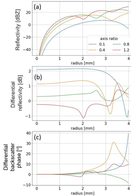
**Figure 8.** Simulated (a) radar reflectivity, (b) differential reflectivity and (c) differential backscatter phase for spheroids with different axis ratios as a function of maximum radius at 35 GHz with  $45^\circ$  looking angle. All spheroids have ice fraction of 0.6 and zero mean canting angle.
