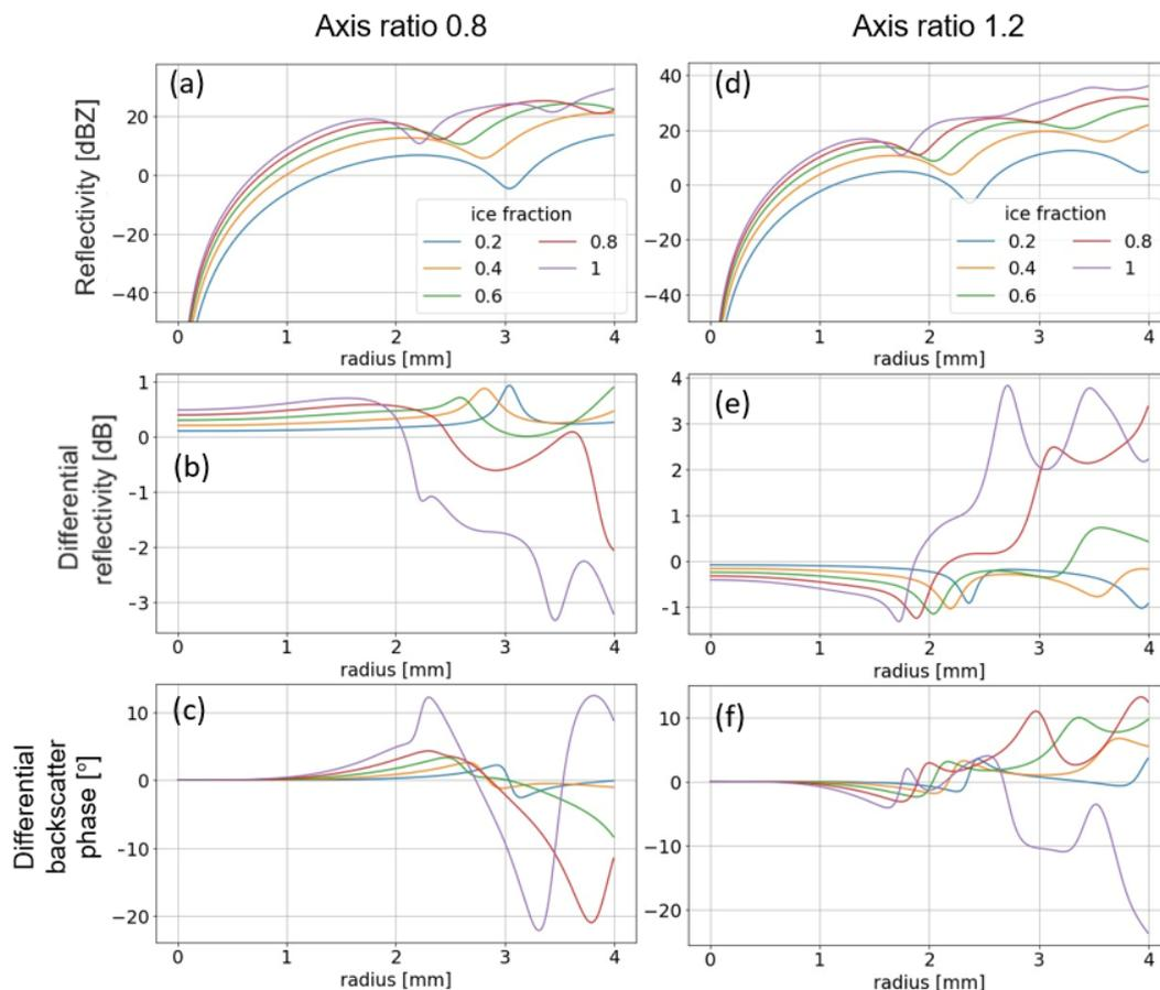
**Figure 9.** Simulated radar variables for spheroids with zero mean canting angle and different ice fractions as a function of maximum radius at 35 GHz with  $45^\circ$  looking angle. Panels (a-c) show the radar reflectivity, differential reflectivity and differential backscatter phase for spheroids with fixed axis ratio of 0.8. Panels (d-f) show the same for spheroids with fixed axis ratio of 1.2.
