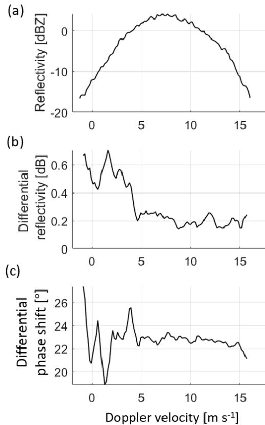
**Figure 28.** (a) Spectral reflectivity, (b) differential reflectivity and (c) differential phase shift at 10003 m at 17:22:57 UTC. Note that the Doppler velocity decreases when the maximum dimension increases.
