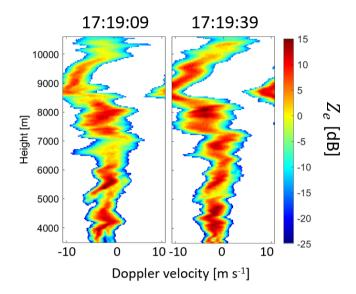
Figure 23. Spectral reflectivity at 17:19:09 and 17:39:39 UTC.
