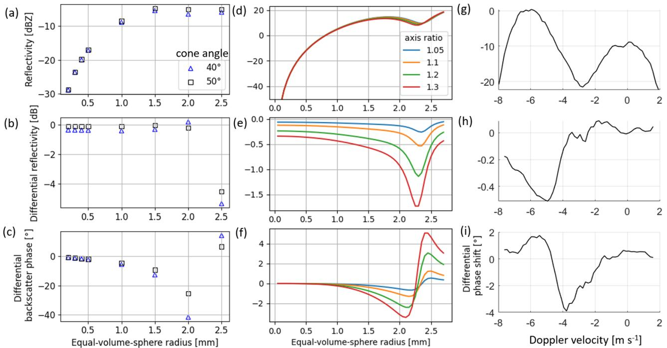
**Figure 25.** Simulated reflectivity, differential reflectivity and differential backscatter phase of conical graupel by Lu et al. (2016) (a-c) and T-matrix method (d-f). (g-i) Spectral reflectivity, differential reflectivity and differential phase shift at 5021 m at 17:22:25 UTC. Note that the Doppler velocity decreases towards more negative values when the radius increases.
