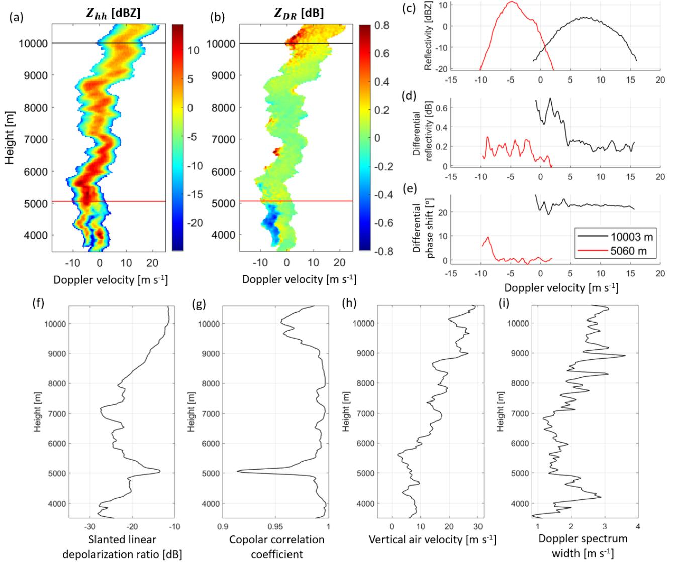
**Figure 26.** 18 June 2021 17:22:57 UTC where the lowest peak of  $SL_{DR}$  and trough of  $\rho_{hv}$  is observed. (a-b) Spectrograms of reflectivity and differential reflectivity (c-e) spectra of reflectivity,  $Z_{DR}$  and  $\Psi_{DP}$  at 5060 m (f-i) profiles of  $SL_{DR}$ ,  $\rho_{hv}$ , vertical air velocity and Doppler spectrum width.
