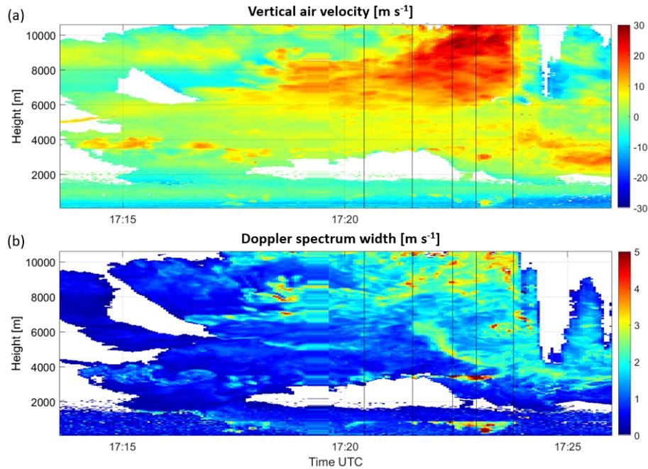
**Figure 20.** (a) Vertical air velocity and (b) Doppler spectrum width of the fourth thunderstorm cloud on 18 June 2021 from 17:14 to 17:26 UTC. Vertical black lines indicate time instants 17:20:26, 17:21:31, 17:22:25, 17:22:57 and 17:23:47 UTC.
