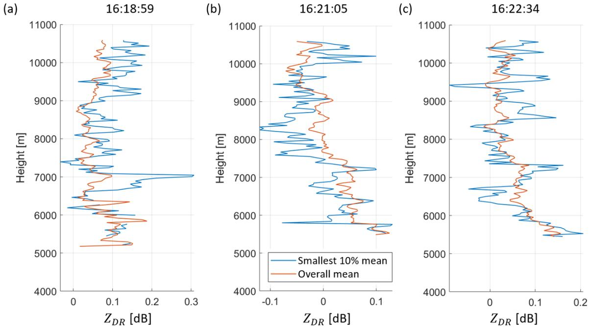
**Figure 13.** Mean  $sZ_{DR}$  of all particles and the smallest 10% of the particles in a radar resolution volume at (a) 18 June 2021 16:18:59 UTC, (b) 16:21:05 UTC and (c) 16:22:34 UTC.
