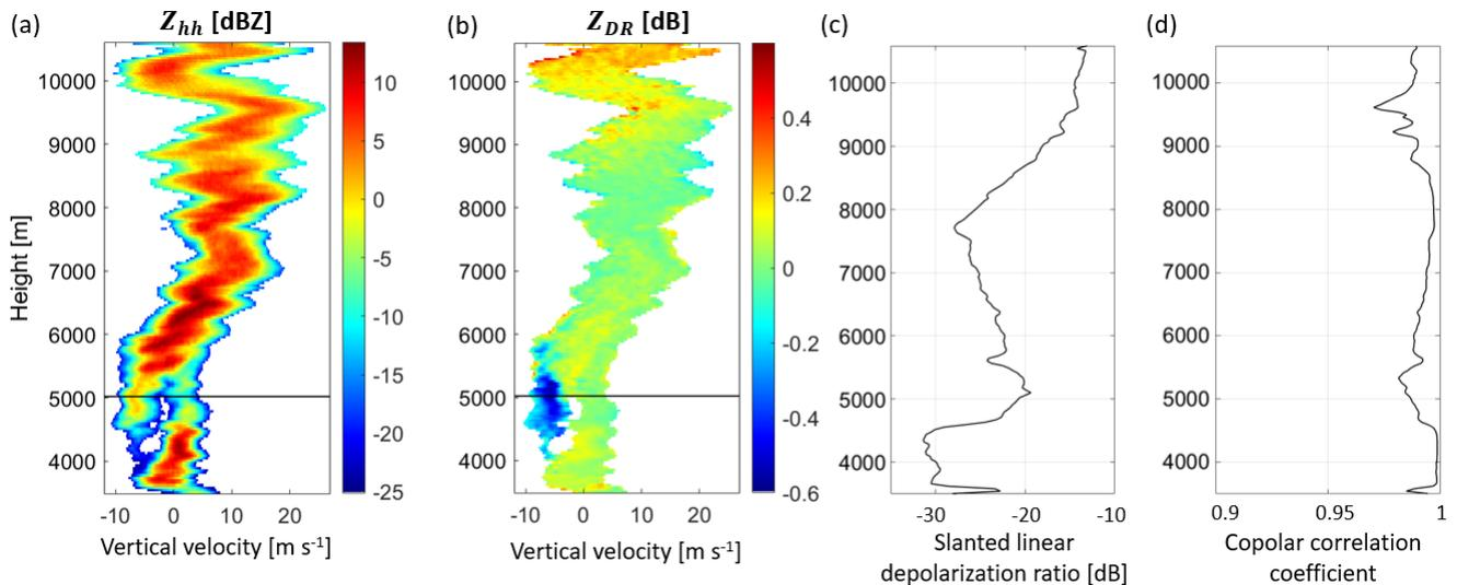
**Figure 24.** Spectrograms of (a) equivalent reflectivity, (b) differential reflectivity, and profiles of (c) slanted linear depolarisation ratio, (d) copolar correlation coefficient at 17:22:25 UTC. Spectra at 5021 m indicated by black horizontal line in (a) and (b) are shown in Fig. 25(g-i).
