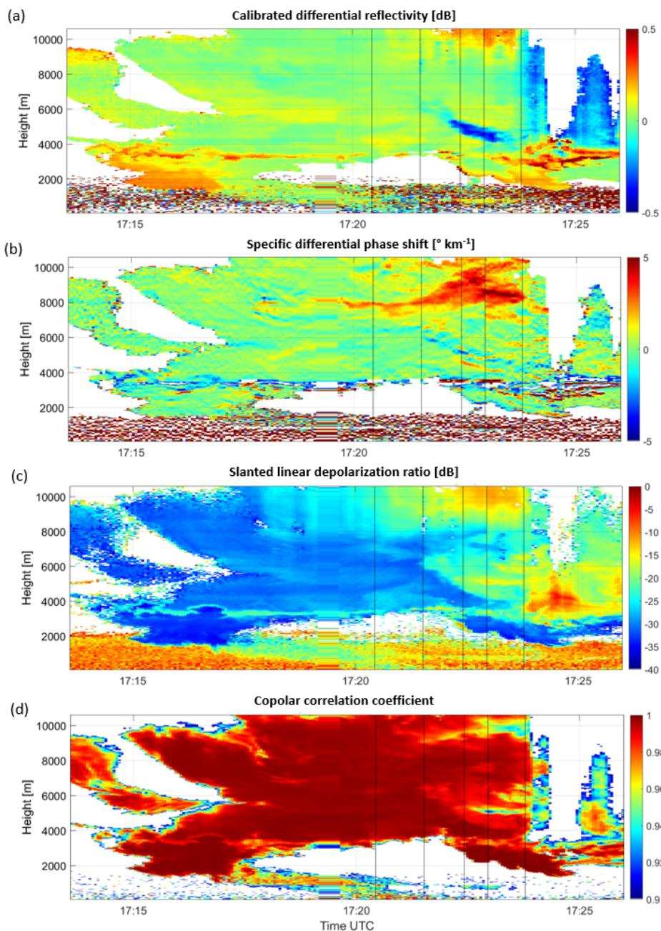
**Figure 19.** (a) Differential reflectivity, (b) specific differential phase shift, (c) slanted linear depolarisation ratio and (d) copolar correlation coefficient of the fourth thunderstorm cloud on 18 June 2021 from 17:14 to 17:26 UTC. Vertical black lines indicate time instants 17:20:26, 17:21:31, 17:22:25, 17:22:57 and 17:23:47 UTC.
