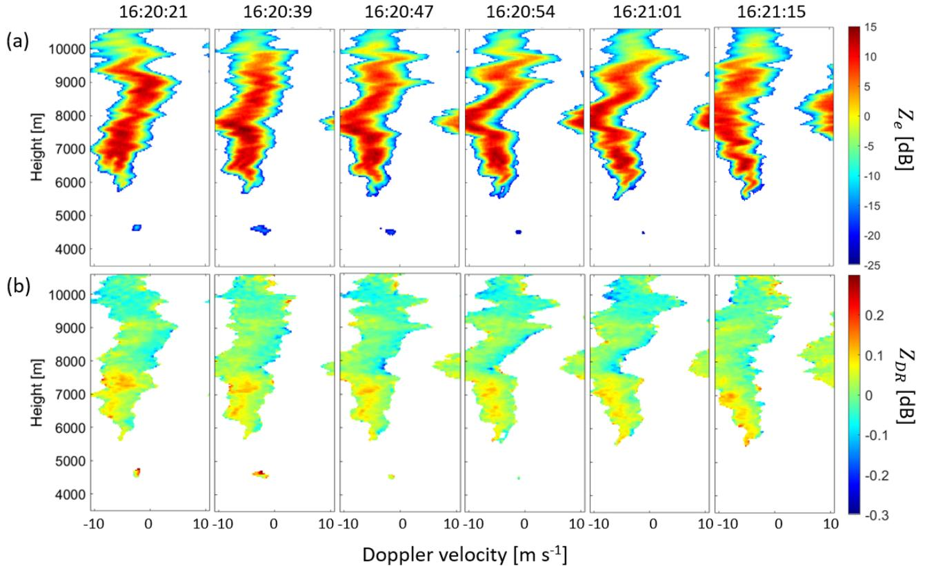
**Figure 16.** (a) Spectral reflectivity and (b) spectral  $Z_{DR}$  on 18 June 2021 from 16:20:21 to 16:21:15 UTC showing presence of supercooled liquid water near 6000 m.
