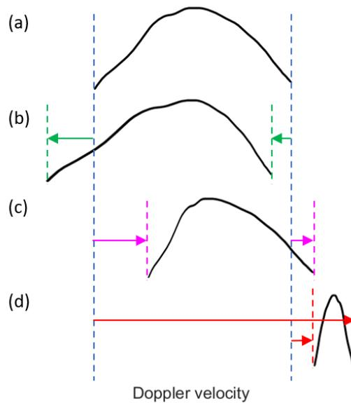
**Figure 14.** A figure to illustrate effects of the sign of vertical wind shear  $s$  on the Doppler spectrum: (a) Doppler spectrum when there is no shear (b) Doppler spectrum widens when  $s$  is negative (c) Doppler spectrum may become narrow when  $s$  is positive (d) Doppler spectrum may flip when  $s$  is positive and  $\frac{sV_t^2}{g}$  is larger than the original spectrum width.
