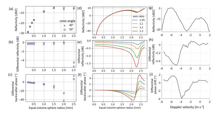
**Figure 24.** Simulated reflectivity, differential reflectivity and differential backscatter phase of conical graupel by Lu et al. (2016) (a-c) and T-matrix method (d-f). (g-i) Spectral reflectivity, differential reflectivity and differential phase shift at 5021 m at 17:22:25 UTC. Note that the Doppler velocity decreases towards more negative values when the radius increases.
