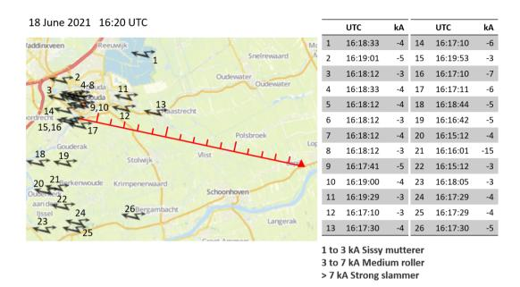
**Figure B1.** Location, time and power of lightning strikes from 18 June 2021 16:15 to 16:20 UTC (© OpenStreetMap contributors 2023. Distributed under the Open Data Commons Open Database License (ODbL) v1.0.)(Kachelmann GmbH). Red triangle shows radar location, red ruler shows line of sight of radar with each mark equal to 1 km.
