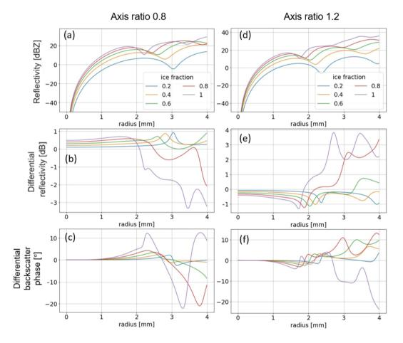
**Figure 9.** Simulated radar variables for spheroids with zero mean canting angle and different ice fractions as a function of maximum radius at 35 GHz with 45° looking angle. Panels (a-c) show the radar reflectivity, differential reflectivity and differential backscatter phase for spheroids with fixed axis ratio of 0.8. Panels (d-f) show the same for spheroids with fixed axis ratio of 1.2.
