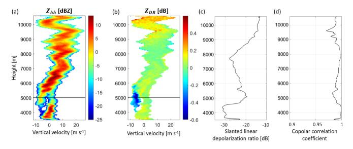
**Figure 23.** <u>Spectrograms Spectrograms of (a) equivalent reflectivity, (b) differential reflectivity, and profiles of (c) slanted linear depolarisation ratio, (d) copolar correlation coefficient at 17:22:25 UTC. Note that the x-axis in (a) and (b) represents the vertical velocity. Spectra at 5021 m indicated by black horizontal line in (a) and (b) are shown in Fig. 24(g-i).</u>
