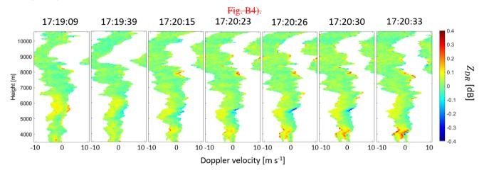
**Figure 22.** Spectral differential reflectivity before and after a strong lightning strike (-18 kA) at 17:20:27 UTC at 5 km cross-range (strike number 92 in Fig. B5).
