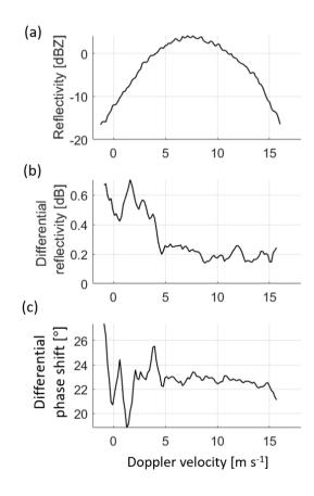
**Figure 27.** (a) Spectral reflectivity, (b) differential reflectivity and (c) differential phase shift at 10003 m at 17:22:57 UTC. Note that the Doppler velocity decreases when the maximum dimension increases.
