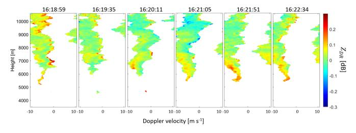
Figure 12. Spectral  $Z_{DR}$  on 18 June 2021 from 16:18:59 to 16:22:34 UTC.
