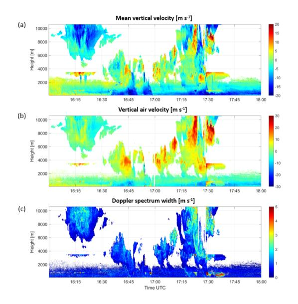
**Figure 5.** (a) Mean vertical velocity, (b) vertical air velocity and (c) Doppler spectrum width on 18 June 2021 16:00 - 17:59 UTC from 35 GHz radar with 45° elevation.
