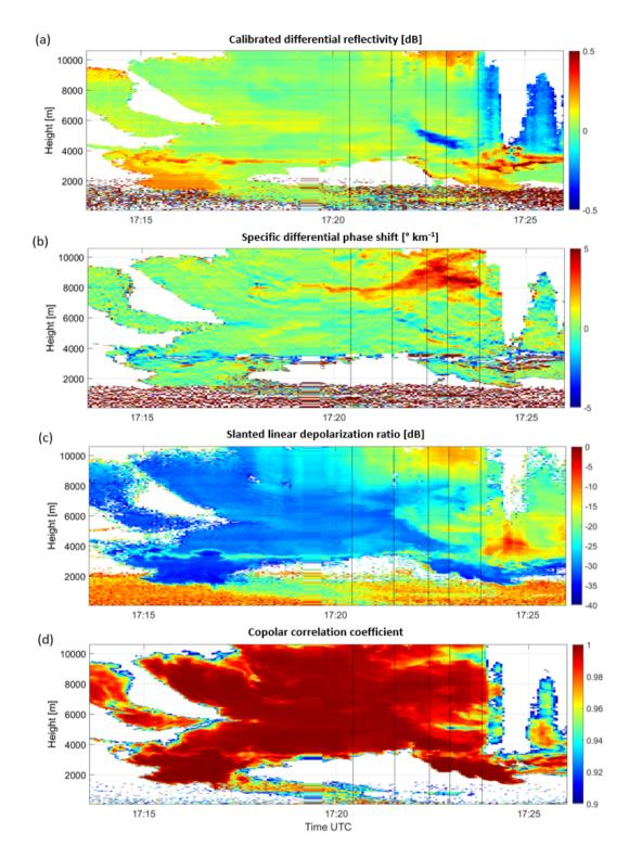
Figure 19. (a) Differential reflectivity, (b) specific differential phase shift, (c) slanted linear depolarisation ratio and (d) copolar correlation coefficient of the fourth thunderstorm cloud on 18 June 2021 from 17:14 to 17:26 UTC. Vertical black lines indicate time instants 17:20:26, 17:21:31, 17:22:25, 17:22:57 and 17:23:47 UTC. 29
