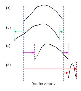
Figure 14. A figure to illustrate effects of the sign of vertical wind shear s on the Doppler spectrum: (a) Doppler spectrum when there is no shear (b) Doppler spectrum widens when s is negative (c) Doppler spectrum may become narrow when s is positive (d) Doppler spectrum may flip when s is positive and  $\frac{sV_t^2}{s}$  is larger than the original spectrum width.
