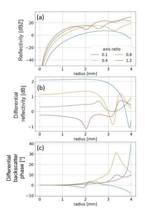
**Figure 8.** Simulated (a) radar reflectivity, (b) differential reflectivity and (c) differential backscatter phase for spheroids with different axis ratios as a function of maximum radius at 35 GHz with 45° looking angle. All spheroids have ice fraction of 0.6 and zero mean canting angle.
