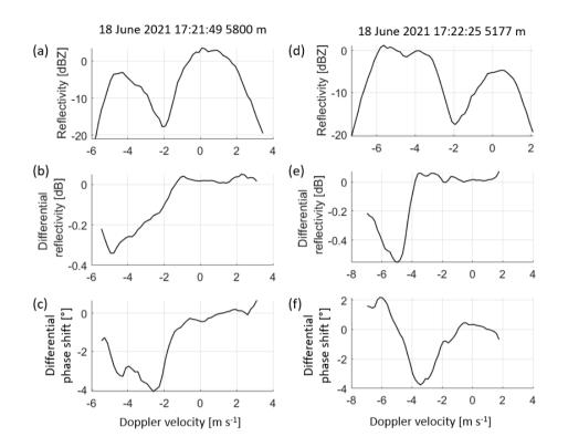
Figure 6. Two examples of Doppler spectra of  $Z_e$ ,  $Z_{DR}$  and  $\Psi_{DP}$  at 35 GHz showing non-Rayleigh scattering.
