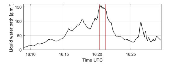
Figure 18. Liquid water path of the first cloud measured at 89 GHz. Time interval from 16:20:21 to 16:21:15 UTC is marked by red lines.
