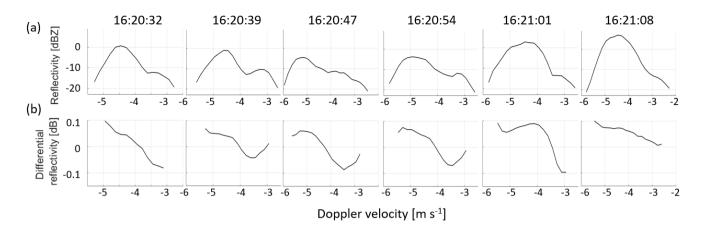
Figure 17. (a) Spectral reflectivity and (b) spectral  $Z_{DR}$  on 18 June 2021 from 16:20:32 to 16:21:08 UTC at 5916 m.
