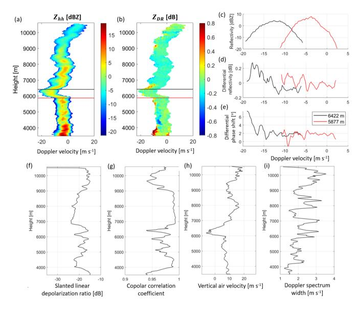
Figure 26. 18 June 2021 17:23:47 UTC where the three peaks of  $SL_{DR}$  and troughs of  $\rho_{hv}$  are observed. (a-b) Spectograms. Spectrograms of reflectivity and differential reflectivity (c-e) spectra of reflectivity,  $Z_{DR}$  and  $\Psi_{DP}$  at 5877 m (middle peak) and 6422 m (highest peak) (f-i) profiles of  $SL_{DR}$ ,  $\rho_{hv}$ , vertical air velocity and Doppler spectrum width.
