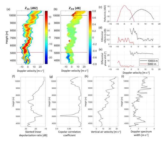
Figure 25. 18 June 2021 17:22:57 UTC where the lowest peak of  $SL_{DR}$  and trough of  $\rho_{hv}$  is observed. (a-b) Spectograms Spectrograms of reflectivity and differential reflectivity (c-e) spectra of reflectivity,  $Z_{DR}$  and  $\Psi_{DP}$  at 5060 m (f-i) profiles of  $SL_{DR}$ ,  $\rho_{hv}$ , vertical air velocity and Doppler spectrum width.
