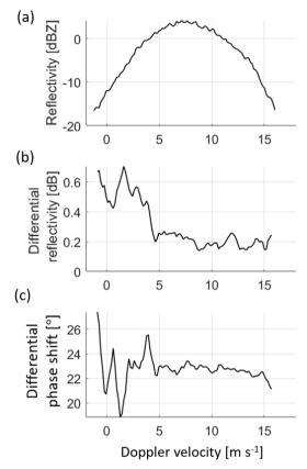
Figure 28. (a) Spectral reflectivity, (b) differential reflectivity and (c) differential phase shift at 10003 m at 17:22:57 UTC. Note that the Doppler velocity decreases when the maximum dimension increases.
