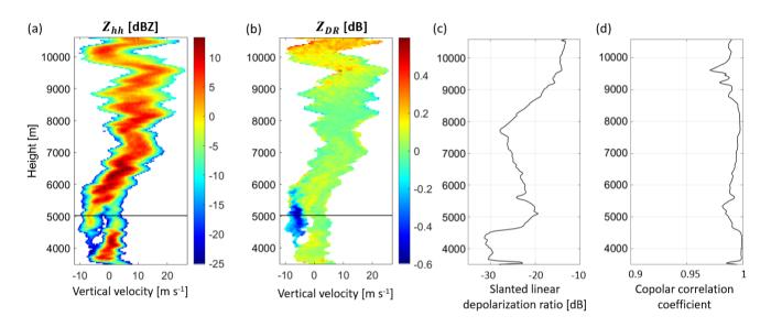
Figure 24. Spectograms of (a) equivalent reflectivity, (b) differential reflectivity, and profiles of (c) slanted linear depolarisation ratio, (d) copolar correlation coefficient at 17:22:25 UTC. Spectra at 5021 m indicated by black horizontal line in (a) and (b) are shown in Fig. 25(d-fg-i).
