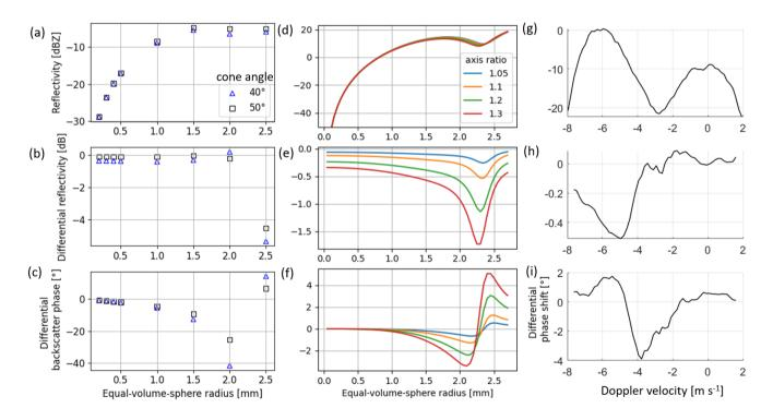
**Figure 25.** Simulated reflectivity, differential reflectivity and differential backscatter phase of conical graupel by Lu et al. (2016) (a-c) and T-matrix method (d-f). (g-i) Spectral reflectivity, differential reflectivity and differential phase shift at 5021 m at 17:22:25 UTC. Note that the Doppler velocity decreases towards more negative values when the radius increases.
