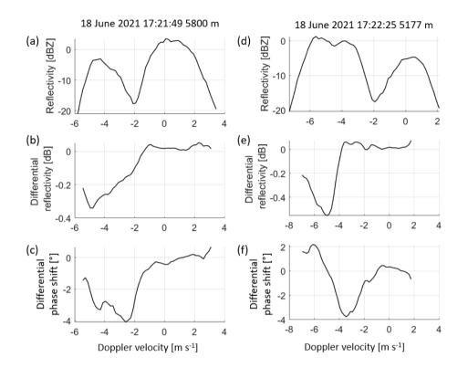
Figure 6. Two examples of Doppler spectra of  $Z_e$ ,  $Z_{DR}$  and  $\Psi_{DP}$  at 35 GHz showing Mie-non-Rayleigh scattering.
