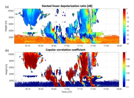
Figure 4. (a)  $SL_{DR}$  and (b)  $\rho_{hv}$  on 18 June 2021 16:00-17:59 UTC.
