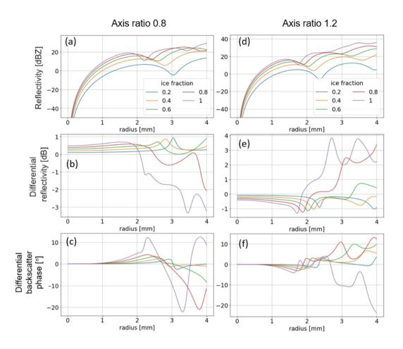
**Figure 9.** Simulated radar variables for horizontally aligned scatterers spheroids with zero mean canting angle and different ice fractions as a function of maximum radius at 35 GHz with 45° looking angle. Panels (a-c) show the radar reflectivity, differential reflectivity and differential backscatter phase for scatterers spheroids with fixed axis ratio of 0.8. Panels (d-f) show the same for scatterers spheroids with fixed axis ratio of 1.2.
