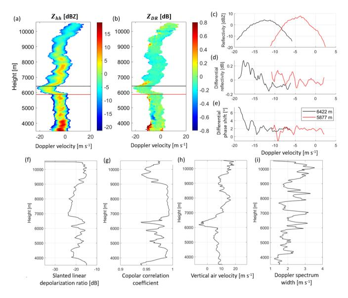
Figure 27. 18 June 2021 17:23:47 UTC where the three peaks of  $SL_{DR}$  and troughs of  $\rho_{hv}$  are observed. (a-b) Spectograms of reflectivity and differential reflectivity (c-e) spectra of reflectivity,  $Z_{DR}$  and  $\Psi_{DP}$  at 5877 m (middle peak) and 6422 m (highest peak) (f-i) profiles of  $SL_{DR}$ ,  $\rho_{hv}$ , vertical air velocity and Doppler spectrum width.
