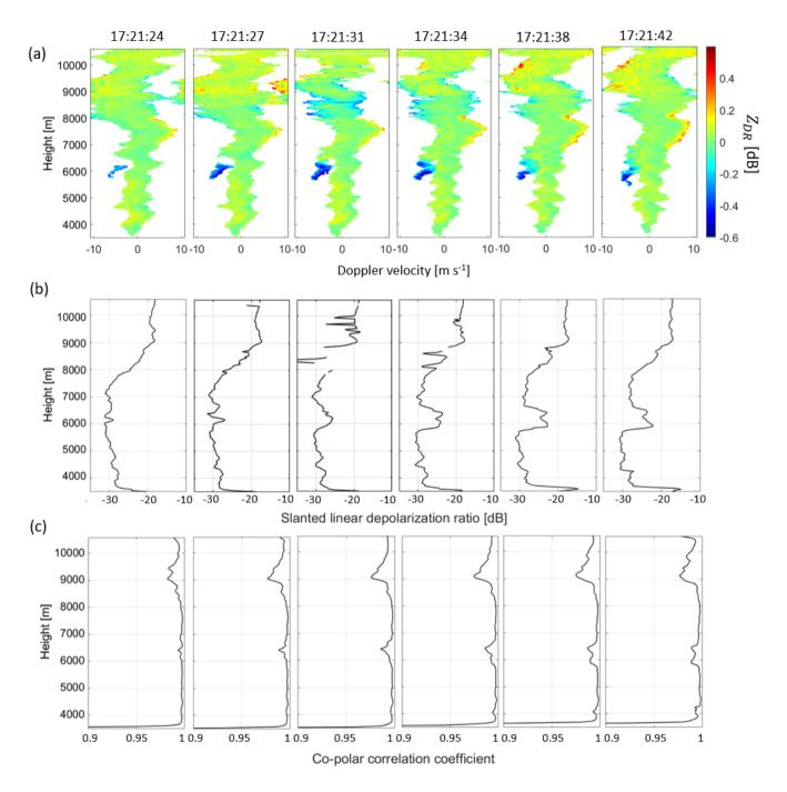
**Figure 21.** (a) Spectral differential reflectivity (b) slanted linear depolarisation ratio and (c) copolar correlation coefficient before and after lightning strike (5 kA) at 17:21:32 UTC on the line-of-sight of the radar between 8000 m and 9000 m (strike number 7 in Fig. B4).
