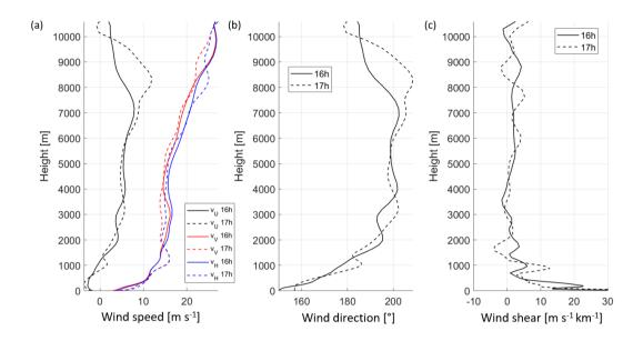
Figure 15. (a) Mean horizontal wind, (b) horizontal wind direction relative to North and (c) vertical wind shear at 18 June 2021 16:00 and 17:00 UTC. These data are outputs of the ECMWF Integrated Forecast System (IFS) over Cabauw (O'Connor, 2022).
