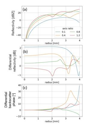
**Figure 8.** Simulated (a) radar reflectivity, (b) differential reflectivity and (c) differential backscatter phase for horizontally aligned scatterers spheroids with different axis ratios as a function of maximum radius at 35 GHz with 45° looking angle. All scatterers spheroids have ice fraction of 0.6 and zero mean canting angle.
