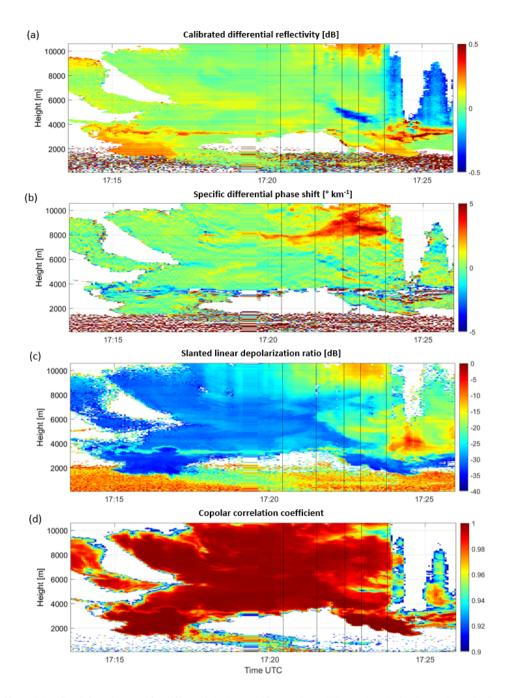
**Figure 19.** (a) Differential reflectivity, (b) specific differential phase shift, (c) slanted linear depolarisation ratio and (d) copolar correlation coefficient of the fourth thunderstorm cloud on 18 June 2021 from 17:14 to 17:26 UTC. Vertical black lines indicate time instants 17:20:26, 17:21:31, 17:22:25, 17:22:57 and 17:23:47 UTC.
