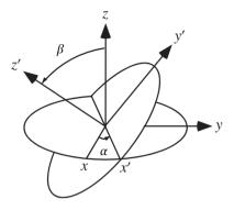
**Figure 7.** Definition of Euler angles  $\alpha$  and  $\beta$ . The *xyz* coordinate frame has the *z* axis aligned with the radar's zenith direction. The rotated frame is denoted as x'y'z', corresponding to the particle's orientation. Starting from the *xyz* frame, a rotation by angle  $\alpha$  around the *z* axis results in the intermediate frame  $x'y_1z$ . This is followed by a rotation by angle  $\beta$  around the *x'* axis to achieve the final x'y'z' frame.
