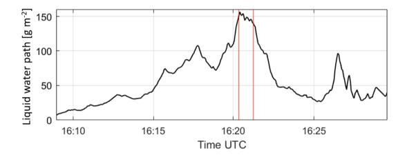
Figure 18. Liquid water path of the first cloud measured at 94-89 GHz. Time interval from 16:20:21 to 16:21:15 UTC is marked by red lines.
