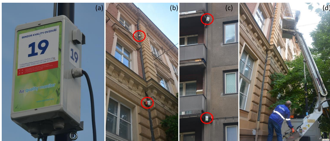
Figure 2. Photos of LCSs deployed in the Legerova campaign (Prague, Czech Republic). (a) The detailed picture of LCS stations used for monitoring of NO 2 , O 3 , PM 10 and PM 2.5 concentrations; (b) and (c) installation of LCSs at two different height levels at the Sokolská school location and Legerova location; (d) picture of the lift platform used for installation of LCSs.
