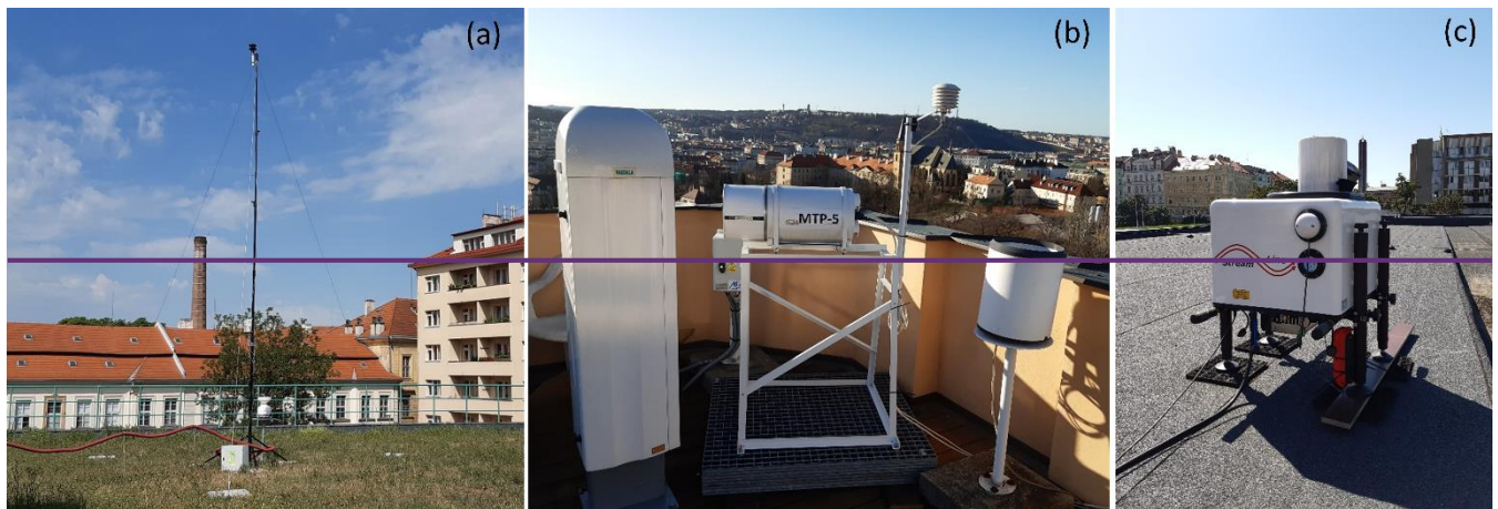
Figure. 4. Supplementary non-reference meteorological measurement used for TURBAN observation campaign: (a) mobile telescopic meteorological mast (MM, height 7.5 m) installed in PVK garden, (b) microwave radiometer MTP 5 He (MWR; for temperature profile measurement up to 1 km height) placed at the Karlov MS; (c) Doppler LIDAR StreamLine XR (for wind and backscatter intensity measurement up to 1.2 km height) placed at the PVK roof.
