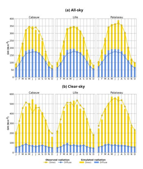
**Figure 4.** Comparisons of the monthly means (2010-2020) of measured (lines) and simulated in hindcast mode (columns) daytime average (a) all-sky and (b) clear-sky irradiances for the three irradiance measurements stations of the BNF region. The total height of each column or line represents the monthly average global irradiance, which is the sum of the direct (in yellow) and diffuse (in blue) components.
