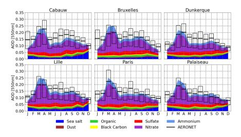
**Figure 5.** Comparisons of the monthly means (2010-2020) of AOD at 550 nm simulated by ALADIN in hindcast mode (colored areas) with coincident photometric measurements (black boxes) for the six AERONET measurement sites located in the BNF region. The boundaries of the boxes correspond to the first and third quartiles (i.e. 25 and 75%), respectively, while the thick black lines inside of each box represent the associated monthly averages.
