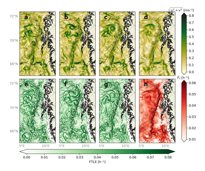
**Figure 6.** a, b and c) Velocity fields from three different Barents-2.5 EPS ensemble members at the LoVe region at 2023-02-02 00:00 and d) ensemble averaged velocity field over all EPS members. e, f and g) Backwards FTLE fields computed over 2023-02-01 for the members shown in a, b and c. h) The ensemble-averaged FTLE field. Bathymetric contours are indicated with gray dashed lines
