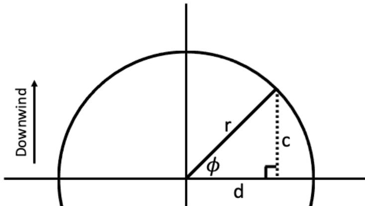
25 **Supplemental Figure 3: Illustration of the geometric relations between variables necessary for estimating a cold pool candidate's radius.**
