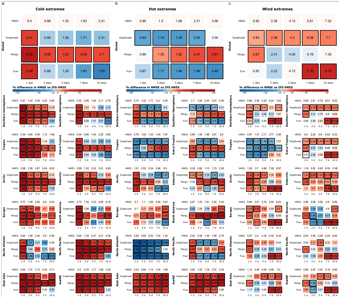
Figure D3. RMSE scorecard for cold (a) as in Figure 3, hot (b) but using ERA5 as ground truth for the data-driven forecasts and wind extremes (c) IFS HRES at a global and regional scale, computed on time 0 as ground truth for the (a) 1%-lowest 2m temperature, (b) 1%-highest 2m temperature and (c) 1%-highest 10m windspeed observations, respectively IFS HRES forecasts.
