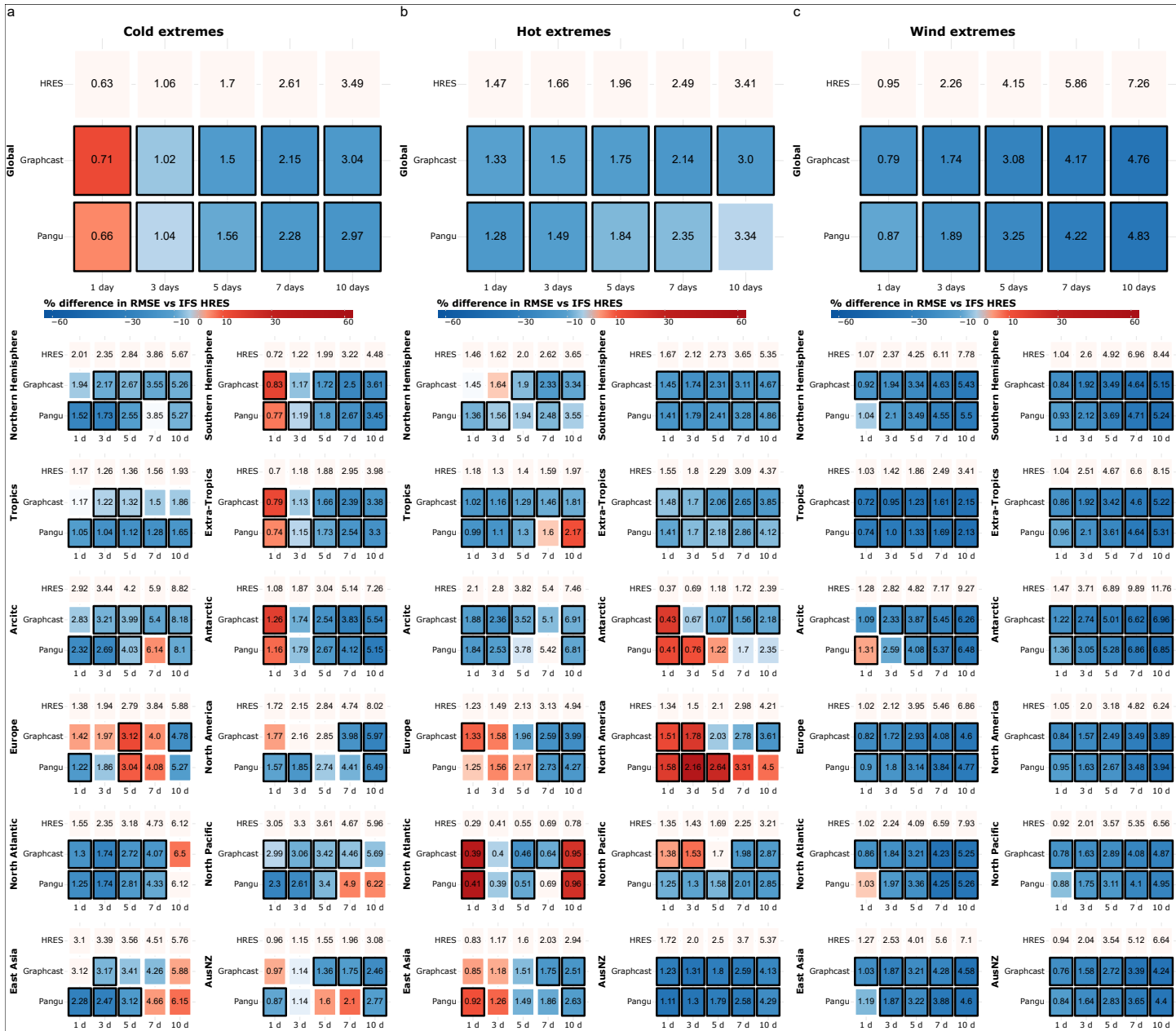
Figure C2. RMSE scorecard for cold (a), hot (b) and wind extremes (c) at a global and regional scale, computed on the (a) 1% lowest 2m temperature, (b) 1% highest 2m temperature and (c) 1% highest 10m windspeed data-points, respectively, selected on the basis of the IFS HRES forecast. Black borders indicate statistically significant differences in performance from IFS HRES, at the 5% level.
