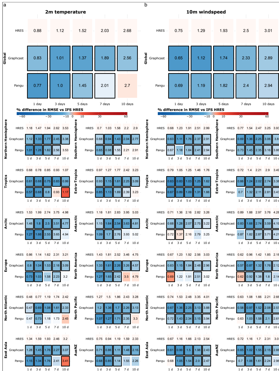
Figure 1. RMSE scorecard for 2m temperature (a) and 10m windspeed (b) at a global and regional scale, computed on all test observations data-points . Blue shades indicate better performance than IFS HRES, red shades worse performance. Black borders indicate significantly different performance from IFS HRES, at the 5% level.
