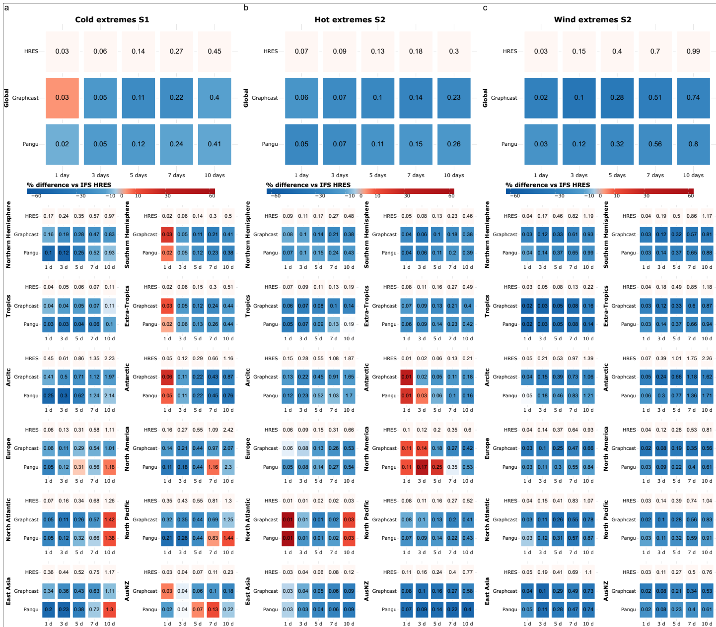
Figure B1. Scorecard for a) cold, b) hot and c) windy extremes based on rectangular partitions with a) 5th and b-c) 95th quantile of all test data-points in the given region as cut-off values. Blue shades indicate better performance than IFS HRES, red shades worse performance.
