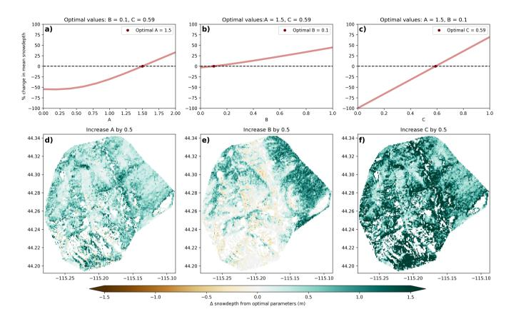
Figure B1. Percent change in scene-wide mean snow depth with varying A, B, and C parameters from optimized values (A = 1.5, B = 0.1, C = 0.59) for the Banner Summit 2021 site (a-c). Changes in S1 snow depth retrievals when increasing each parameter by 0.5 from the optimal value and keeping the other parameters at their optimal value (d-f).
