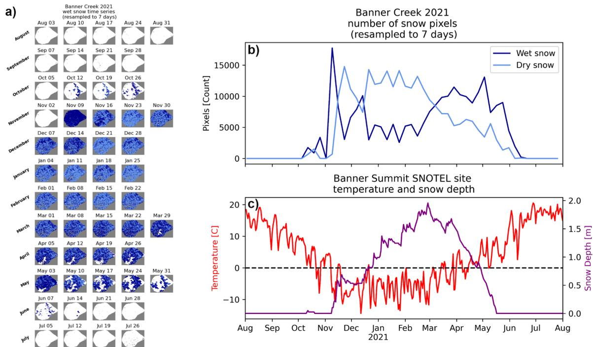
**Figure B3.** Time series of snow classifications for the 2020-2021 winter at the Banner study site (a) with no snow (white), dry snow (light blue), wet snow (dark blue). Number of dry vs. wet snow pixels in the scene from August 2020 to August 2021 (b), and temperature and snow depth values from the Banner Summit SNOTEL (c).
