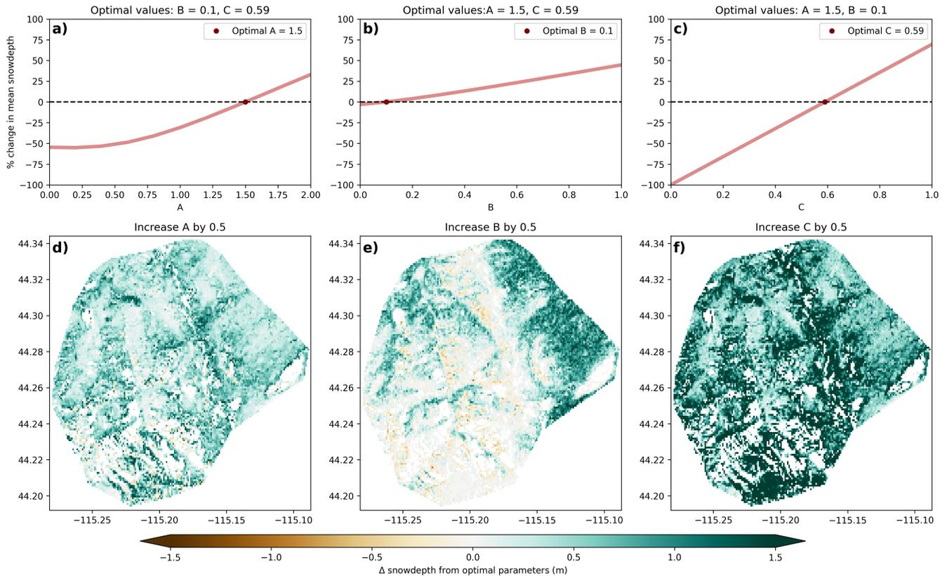
**Figure B1.** Percent change in scene-wide mean snow depth with varying  $A$ ,  $B$ , and  $C$  parameters from optimized values ( $A = 1.5$ ,  $B = 0.1$ ,  $C = 0.59$ ) for the Banner Summit 2021 site (a-c). Changes in S1 snow depth retrievals when increasing each parameter by 0.5 from the optimal value and keeping the other parameters at their optimal value (d-f).
