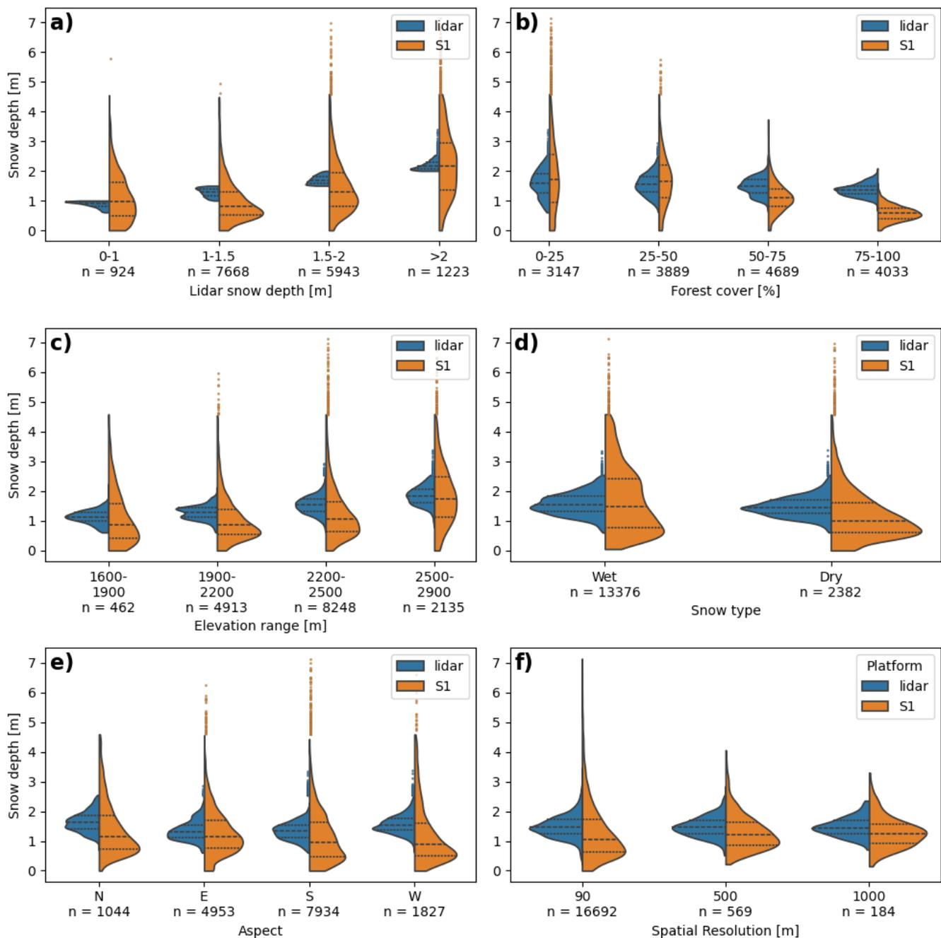
**Figure 5.** Distributions of lidar and retrieved snow depths at Banner 2021 subset by a) snow depth, b) FC, c) elevation, d) wet vs. dry snow, e) aspect, and f) spatial resolution. Values between the 1st–99th percentiles are incorporated into the distributions, while outliers beyond this range are indicated with blue or orange points. Dashed lines indicate the 25th, 50th, and 75th percentiles.
