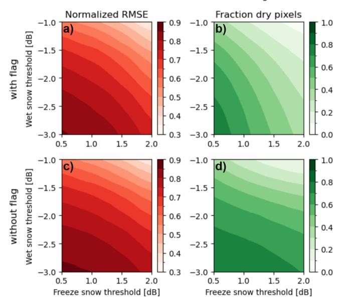
**Figure B2.** Binned mean normalized RMSEs (a & c) and fraction of dry pixels (b & d) for permutations of the newly wet and freezing thresholds and with (top row) and without (bottom row) the alternative wet snow flagging for the Banner 2021 lidar flight.
