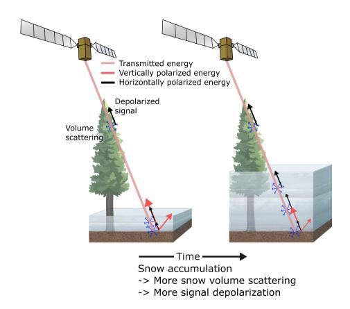
**Figure 1.** Idealized conceptual figure showing the increases in cross-polarized backscatter relative to co-polarized backscatter with increasing snow depth.
