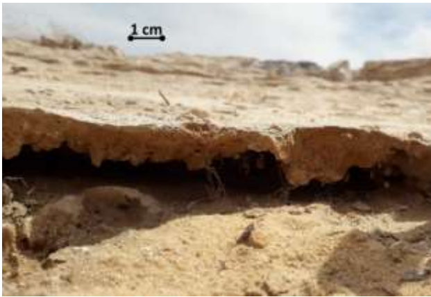
Figure 8: Thin and brittle crust of gypsum that formed over the contaminated sandy soils.
