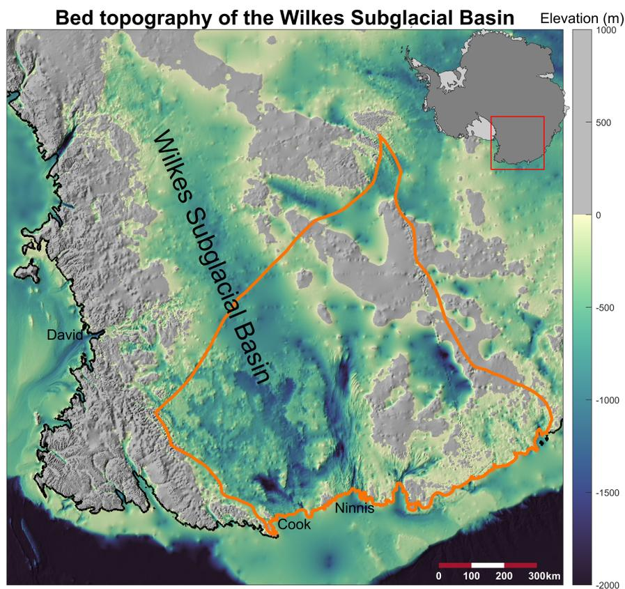
**Figure 1.** Bed topography of the Wilkes Subglacial Basin (WSB) and the designated catchment used as the model domain. The three primary outlet glaciers of the WSB, (Cook, Ninnis and David glaciers) are marked. The orange contour delineates the model domain in this study.
