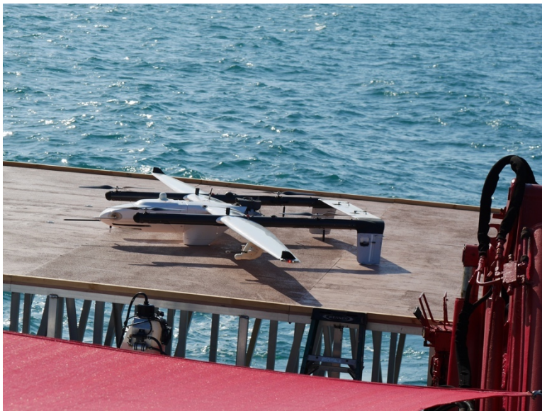
370 Figure 5. FVR-55 with the Clear Sky payload onboard on the 6 x 6 m launch pad on the rear deck of the 371 TowBoatU.S. Richard L. Becker.
