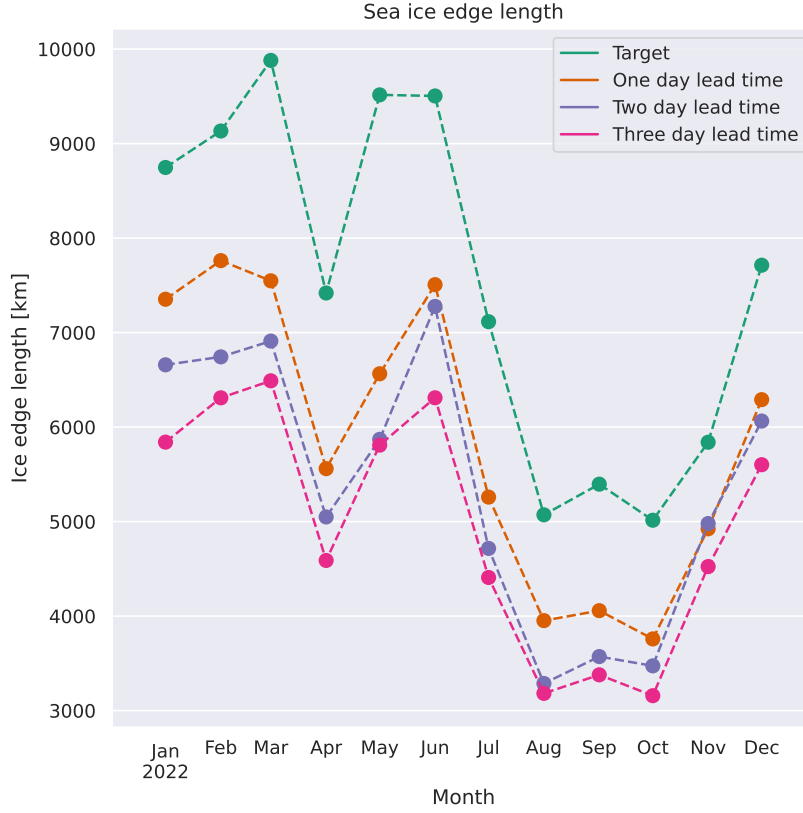
Figure 7. Mean monthly sea ice edge length for 2022, with the sea ice edge defined by a 10% concentration threshold. The considered products are the ice charts and deep learning system for 1 – 3 day lead times.
