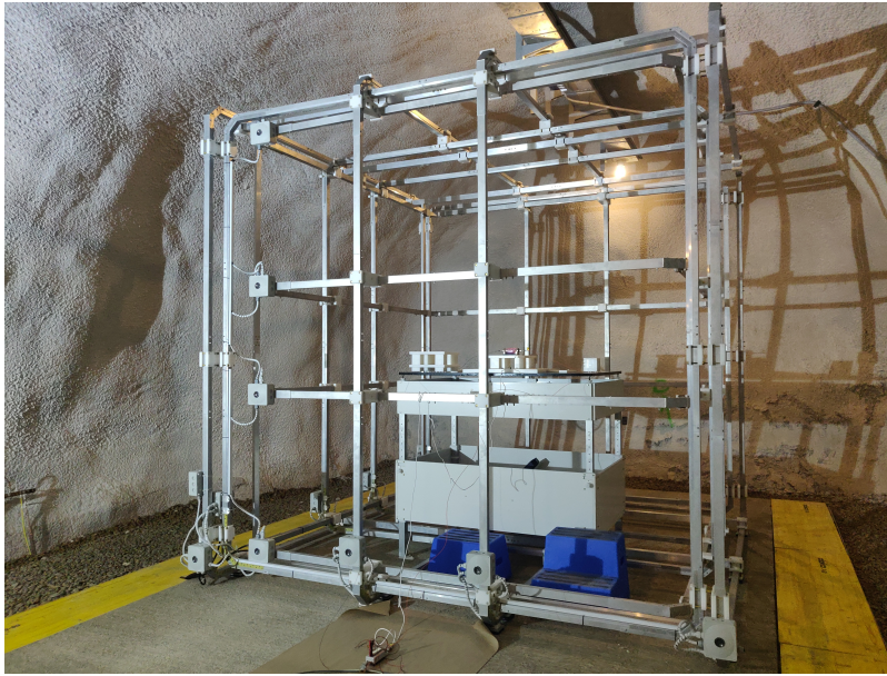
Figure 5. Picture of the Merritt coil system within the tunnel of the Conrad observatory. The side length of the cubic coil system is about 3 m. Each axis has two coil pairs with equal dimensions. This increases the homogeneity of the magnetic field and simplifies the handling of test setups.
