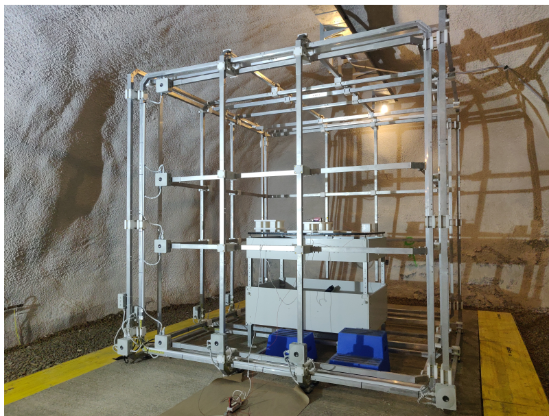
Figure 5. Picture of the Merritt coil system within the tunnel of the Conrad observatory. The side length of the cubic coil system is about 3 m. Each axis has two coil pairs with equal dimensions. This increases the homogeneity of the magnetic field and simplifies the handling of test setups.
