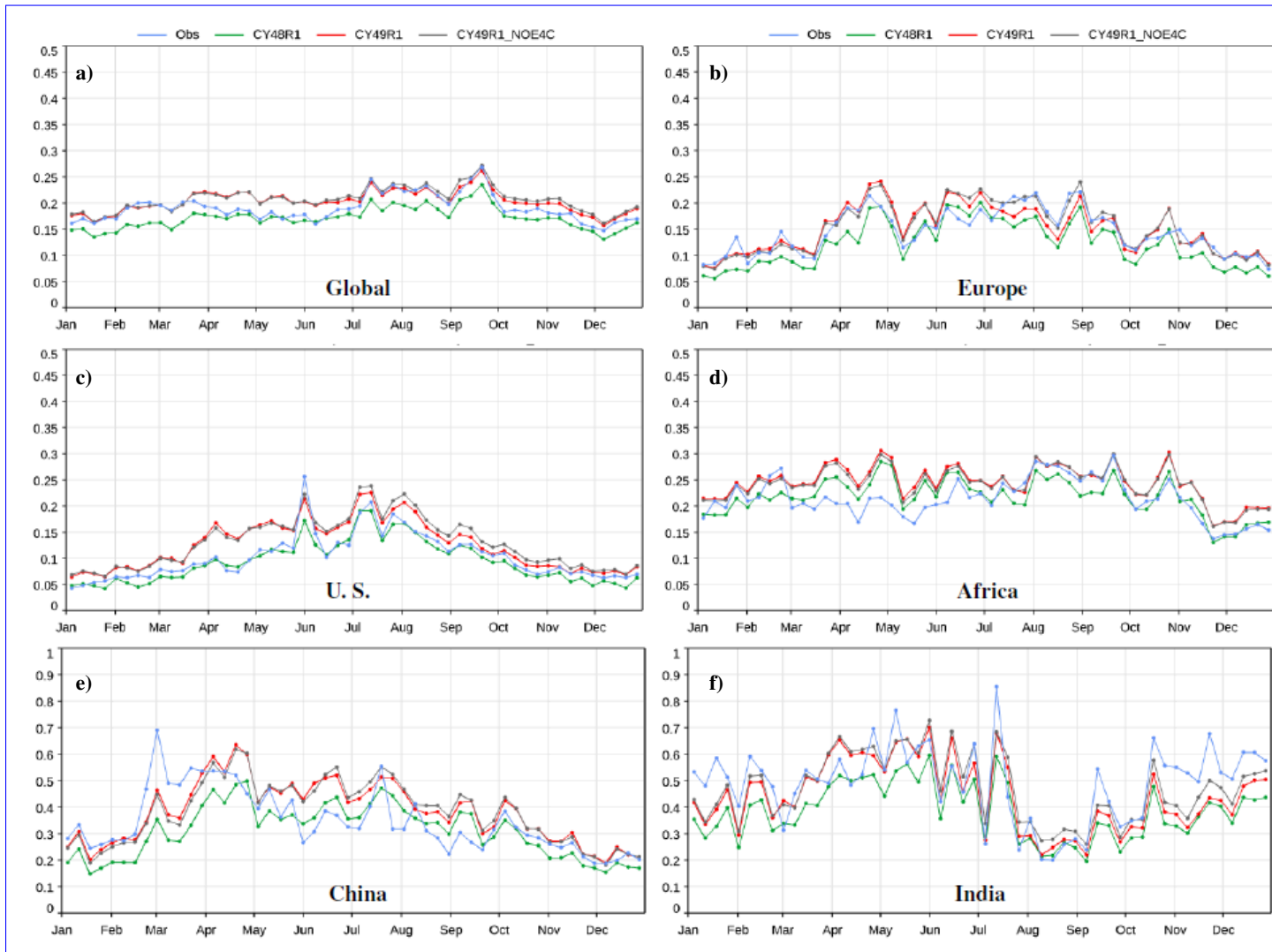
Figure 9. A comparison of the global (panel a, top left) and regional (other panels) weekly simulated and observed AOD (AERONET level 2) at 500nm for 2019. The comparison is made on 461 AERONET sites globally, 113 sites in Europe, 119 sites over the U.S., 68 sites in Africa, 23 in China and 16 in India.
