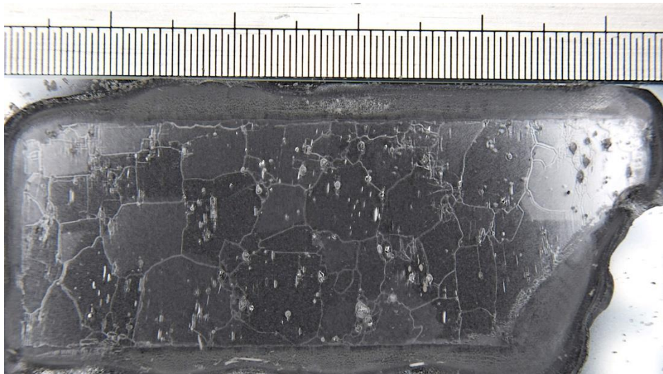
Mosaic on-board camera picture (2x3.8 mm)s from the Cambridge laser system on top. Picture of a 2 x 5 cm sample from ~ 100 ka BP from Skytrain ice core on bottom, grain boundaries and bubbles clearly visible
