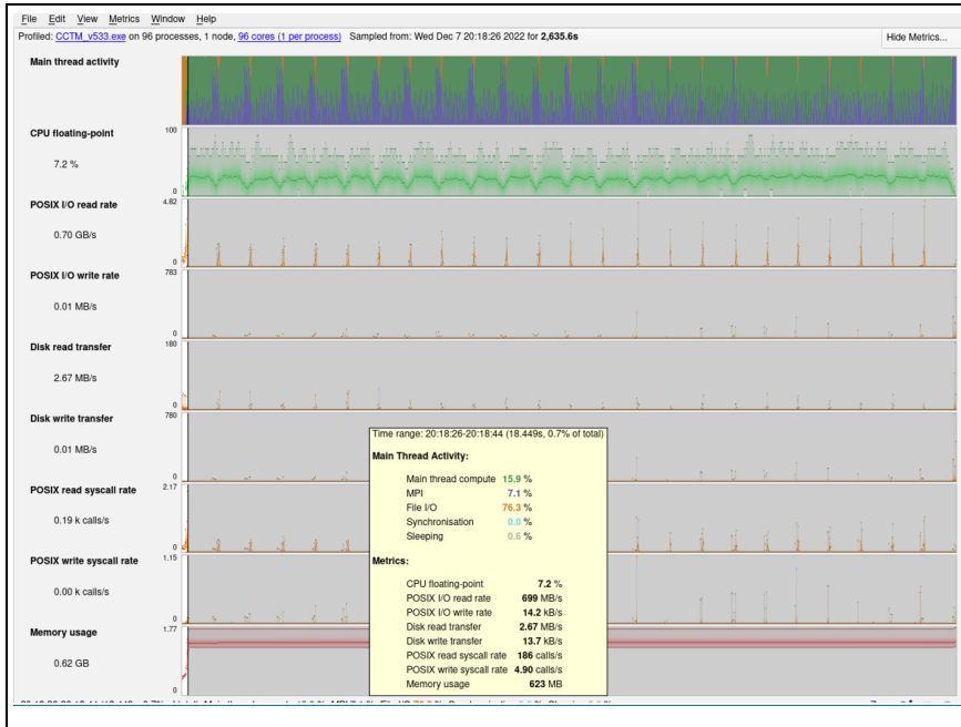
080 Figure A7: ARM MAP™ Code profiler single day performance analysis for Azure's CycleCloud using the Azure Managed Lustre Filesystem.
