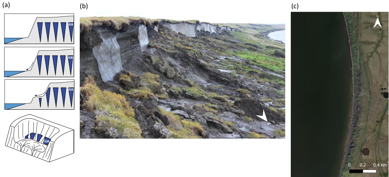
349 350 Figure 6 (a) Scheme of thermoterrace formation, the black arrow indicates the direction of mass movement of thawed material; note 351 that the scheme demonstrates the particular ground ice morphology of a layer with large ice-wedges (adapted from Kizyakov, 2005), 352 but may also consist of other ground ice morphologies. Example of Thermoterraces in Bykovsky Peninsula, NE Siberia, Russia 353 shown (b) on the ground in August 2016 (photo: Alexander Kizyakov) and (c) in a WorldView-2 satellite image from August 2020 354 (ESRI satellite basemap). ESRI basemap used in (c) has the following credits: Esri, DigitalGlobe, GeoEye, i-cubed, USDA FSA, 355 USGS, AEX, Getmapping, Aerogrid, IGN, IGP, swisstopo, and the GIS User Community.
