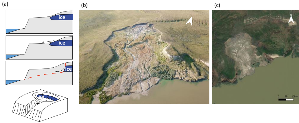
722 723 Figure 7 (a) Scheme of Thermocirque formation, the black arrow indicates the direction of mass movement of thawed material, and 724 the red dotted line stands for the cross-section of the headwall and the slump floor (see Section 3.5). Note that the scheme demonstrates 725 the particular ice morphology of a layer of tabular massive ground ice (adapted from Kizyakov, 2005), but may also consist of other forms 726 of ice-rich ground. Example of a thermocirque in Central Yamal, Russia show on (b) in a UAV photo in August 2019 (photo: Artem 727 Khomutov) and (c) in a WorldView-2 satellite image from July 2018 (Source: ESRI satellite basemap).
