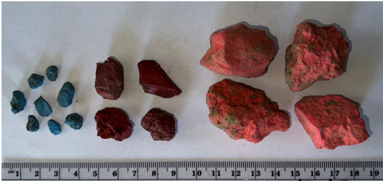
195 Figure 2: Examples of small (left, blue), medium (middle, red), and large (right, pink) experimental particles used in particle drop experiments in Summer 2021 and Spring 2022. Ruler units are in cm.
