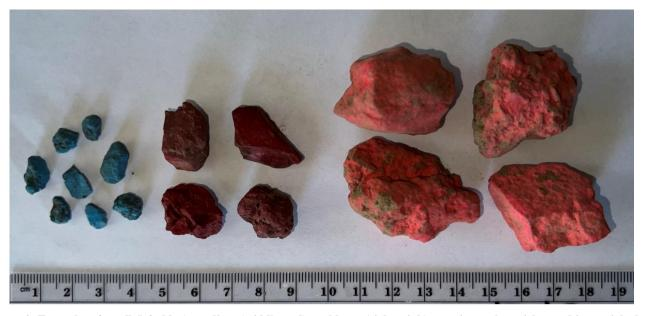
Figure 2: Examples of small (left, blue), medium (middle, red), and large (right, pink) experimental particles used in particle drop experiments in Summer 2021 and Spring 2022. Ruler units are in cm.
