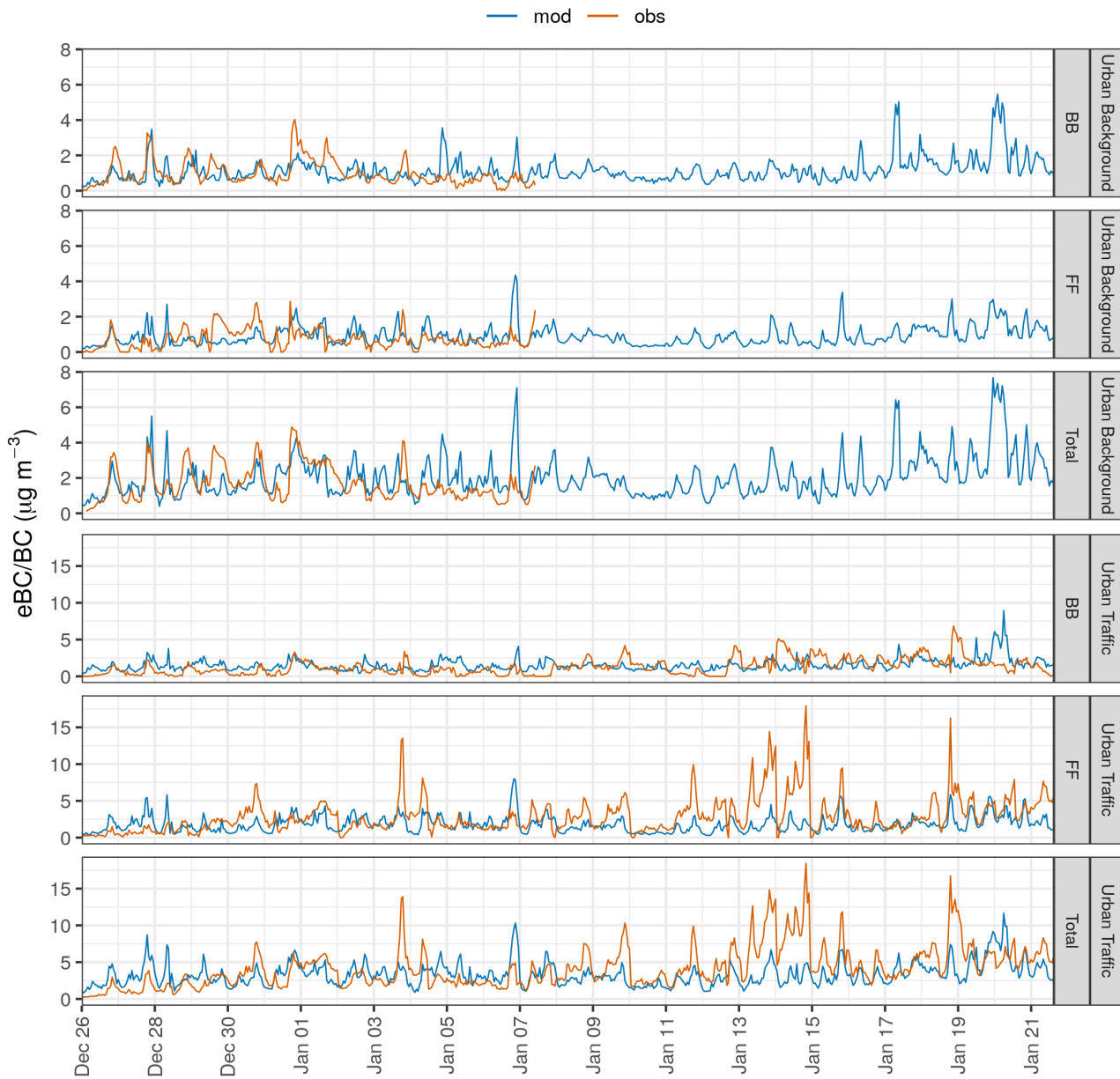
Figure 5. Hourly time series of observed (eBC) and simulated (BC) concentrations at urban traffic and background sites for the period from 26 December 2020 to 21 January 2021. Both simulated and observed concentrations are presented as individual contributions from fossil fuel (FF), biomass burning (BB), and their combined total (Total). Please note the difference in the scale on the y-axis between background and traffic stations.
