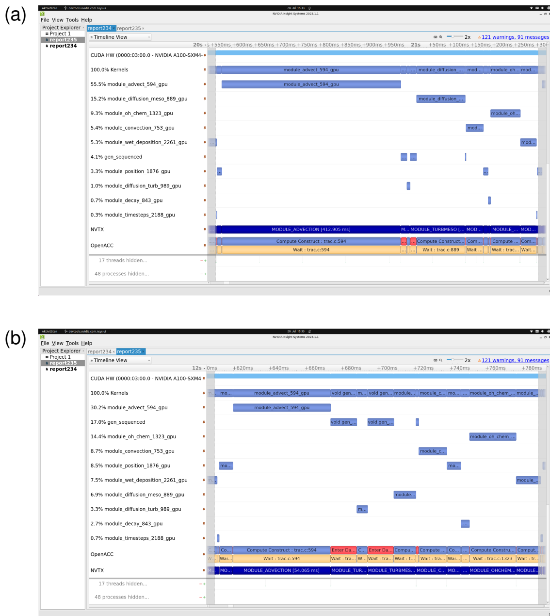
Figure 2. Timeline analyses of a single time step of the MPTRAC Lagrangian transport model for a simulation with 10^8 globally distributed air parcels driven by ERA5 data. Results are shown for (a) the baseline code of MPTRAC and (b) an optimized code version with improved data structures and memory access patterns. The analyses were conducted on the JUWELS Booster HPC system at the Jülich Supercomputing Centre, Germany. The Nsight System report files used to create this figure are made available in the electronic supplement to the paper.
